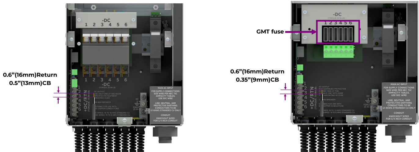
Figure 9 DC Output wiring
