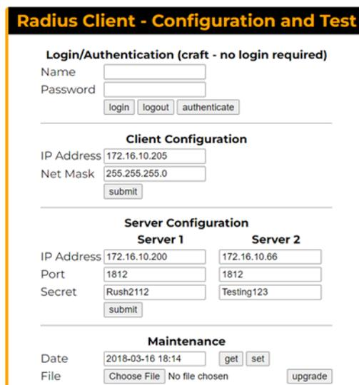
**Figure 11: RADIUS Client Configuration Page**
