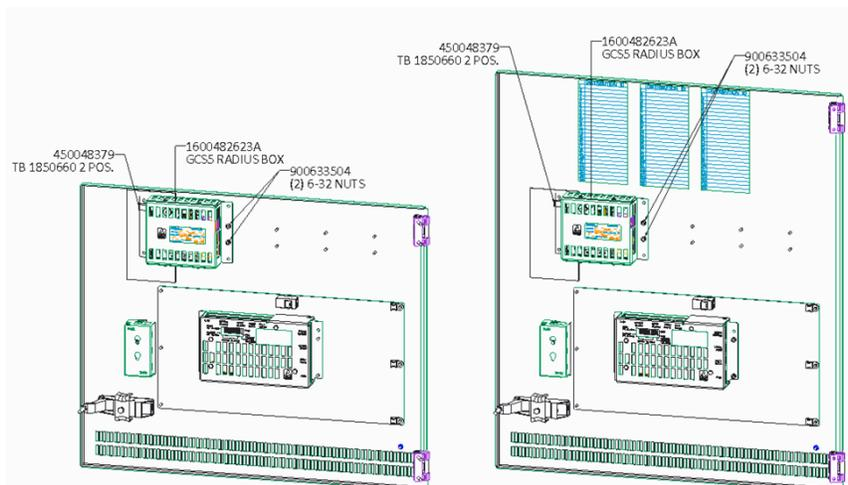
Figure 4: RADIUS Client Installed with Pulsar Plus Controller on Different Infinity-M Distribution Doors
