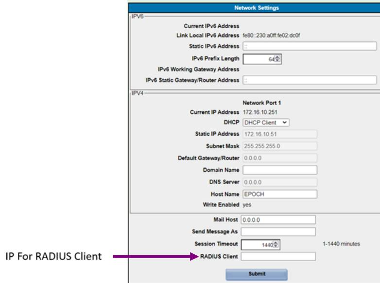
**Figure 11: Configure RADIUS Client IP In Millennium 2**
