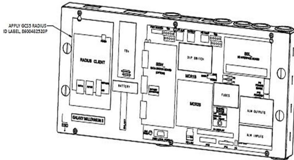
Figure 20: Millennium 2 Lexan Cover With RADIUS Client Identifier Label
