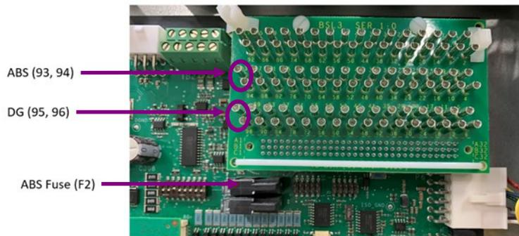
**Figure 7: Millennium 2 BSL3 Alarm Punch-Down (ABS, DG) And ABS Fuse**
