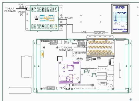
Figure 19: RADIUS Client Network Cable Connections With J85501P1L5
