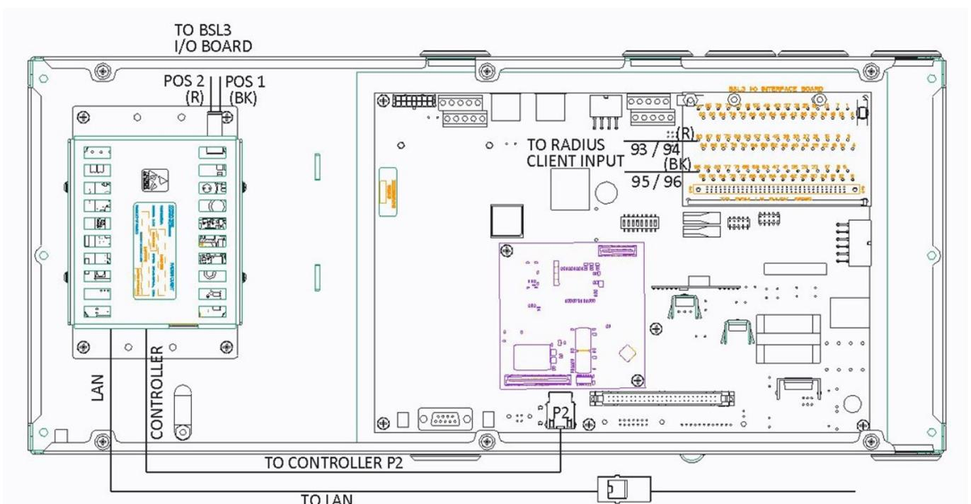
**Figure 13: RADIUS Client Network Cable Connections In J85501P1L1**
