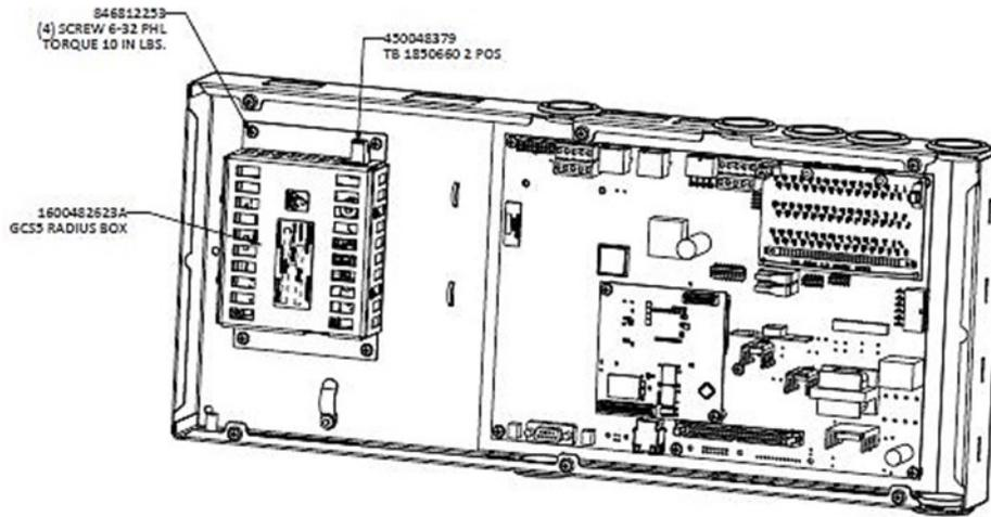
Figure 5: RADIUS Client Installed In J85501P1L1 Millennium 2 Controller Chassis
