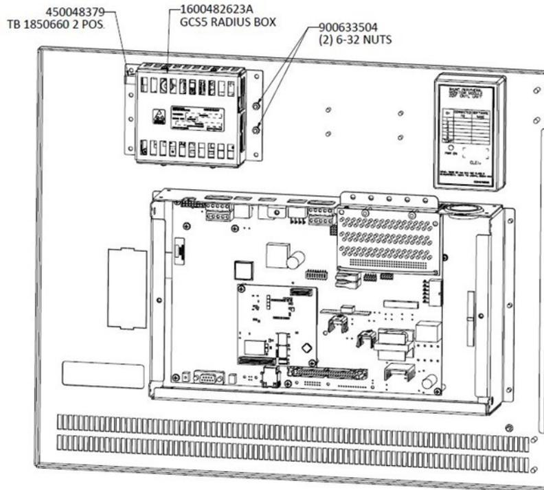
Figure 6: RADIUS Client Installed With J85501P1L5 Millennium 2 Controller In Infinity M
