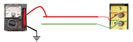
Adjust the meter to read AC voltage and carefully connect the multimeter leads to the RING and TIP terminals for each cable pair connection. If any AC voltage is measure, note the level on Table 1.
