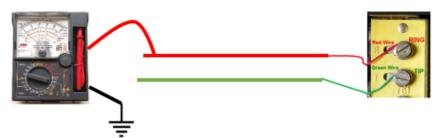
Adjust the meter to read AC voltage and carefully connect the multimeter leads to the RING and GROUND terminals for each cable pair connection. If any AC voltage is measure, note the level on Table 1.
