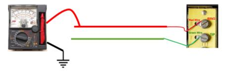
Adjust the meter to the ohms range and carefully connect the multimeter leads to the TIP and GROUND terminals for each cable pair connection. If any resistance is measured > 100K ohms, discard that pair
