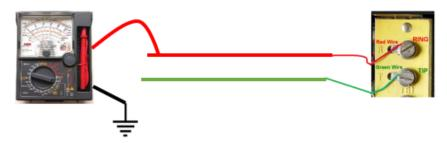
Adjust the meter to the ohms range and carefully connect the multimeter leads to the RING and GROUND terminals for each cable pair connection. If any resistance is measured > 100K ohms, do not use for Line Power.
