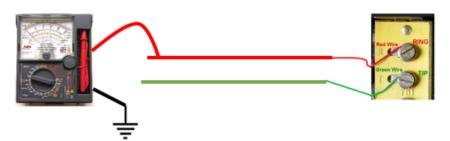
Adjust the meter to read DC voltage and carefully connect the multimeter leads to the RING and GROUND terminals for each cable pair connection. If any DC voltage is measured, record the data in Table 1.
