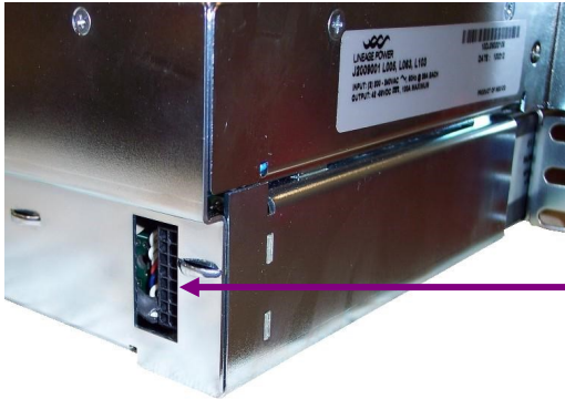
J1 Office Alarm Connector
