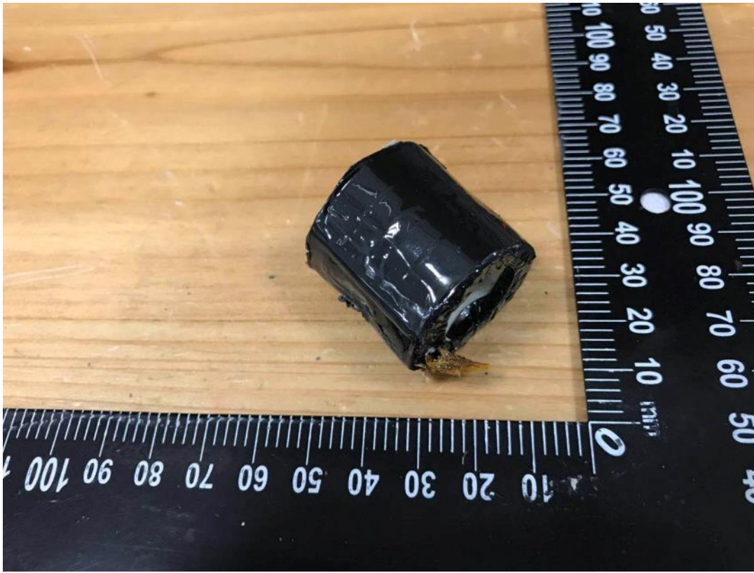
Picture 21 – Transformer T300
