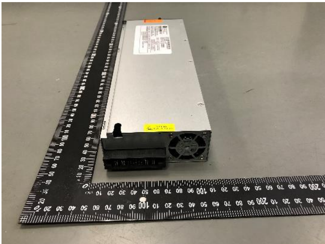
Picture 6 – Overview of Switching Power Supply (Normal airflow and Reverse airflow)
