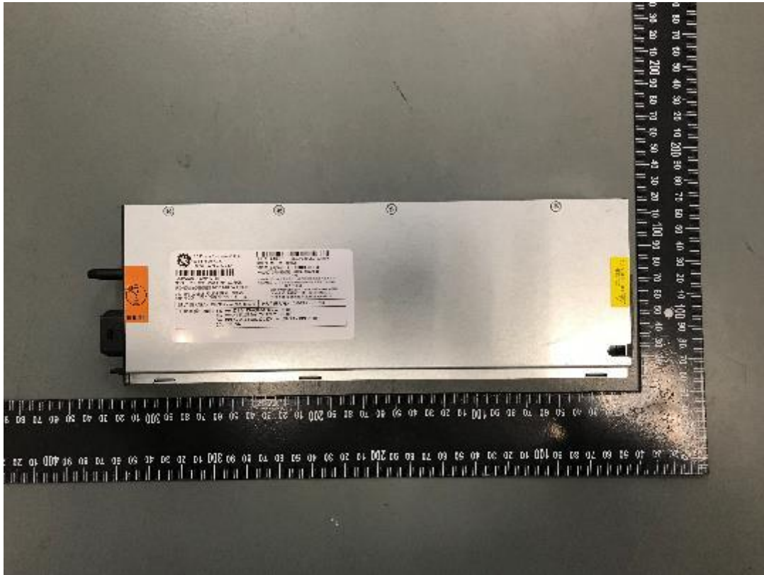
Picture 3 – Overview of Switching Power Supply (Normal airflow and Reverse airflow)
