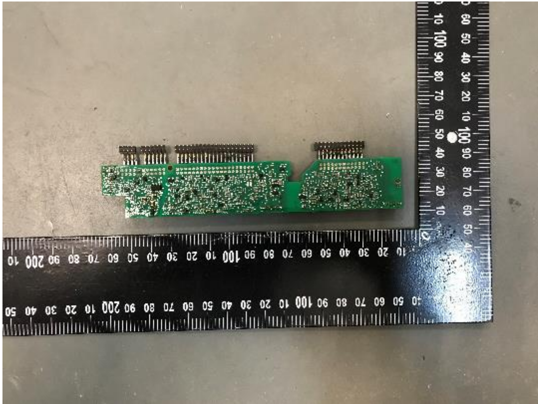
Picture 15 – PWB view of Control Board
