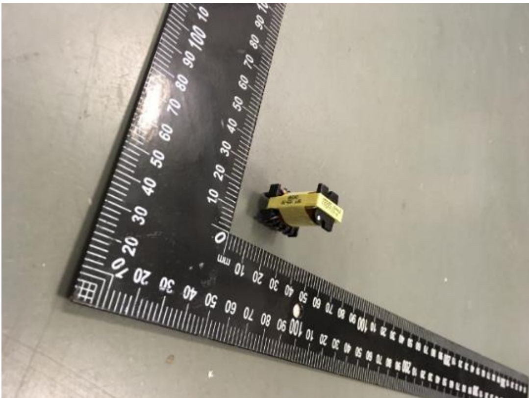
Picture 22 – Transformer view of T700
