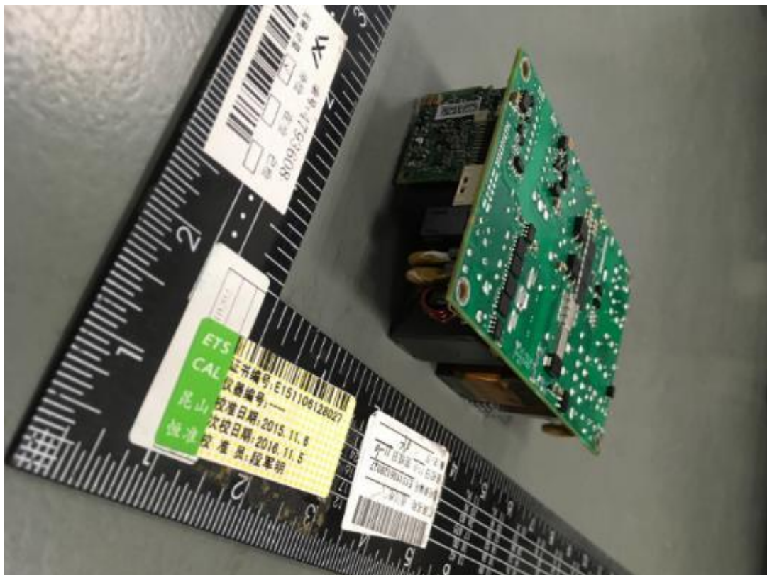
Picture 2 – Overview of Switching Power Supply
