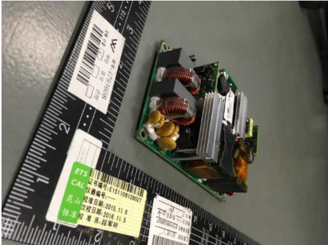
Picture 1 – Overview of Switching Power Supply
