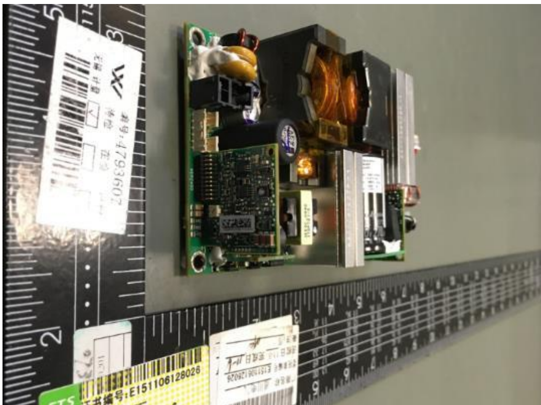
Picture 4 – Overview of Switching Power Supply
