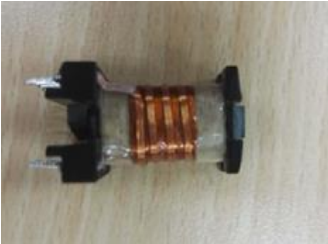
Picture 23 – Winding wire of T700
