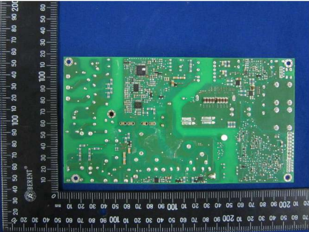
Picture 6 – Trace side view of PCB
