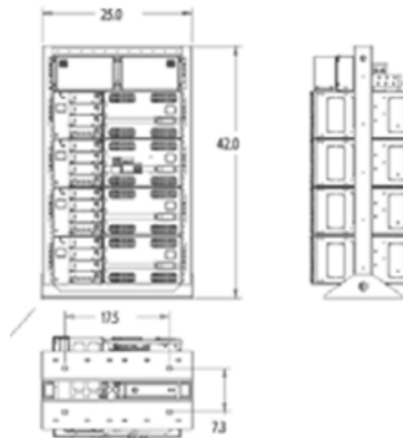
42" high relay rack for mounting 23" wide equipment on a ½ height battery stand or battery stack
