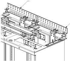
22 sets of 3/8 holes on 1 inch centers for 750 kcmil cable, 7 sets of 1/4 inch holes on 5/8 inch centers
