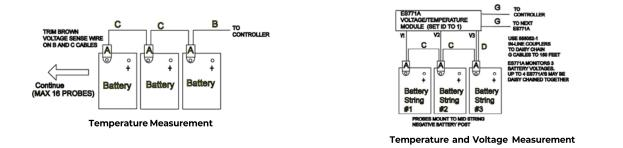
Temperature/Voltage probes are needed for battery monitoring. They are connected to each battery or battery string to provide slope thermal compensation, temperature alarms and voltage imbalance alarms
