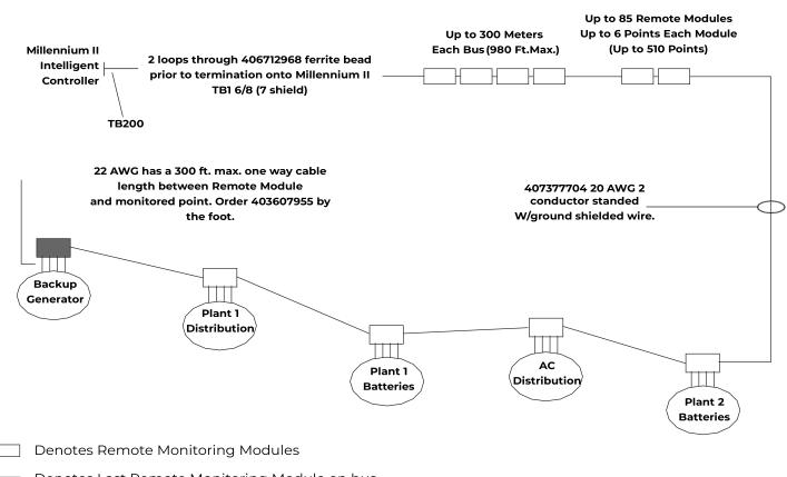
Denotes Last Remote Monitoring Module on bus. A 560 ohm, 10 watt Terminating Resistor is required for proper operation.
