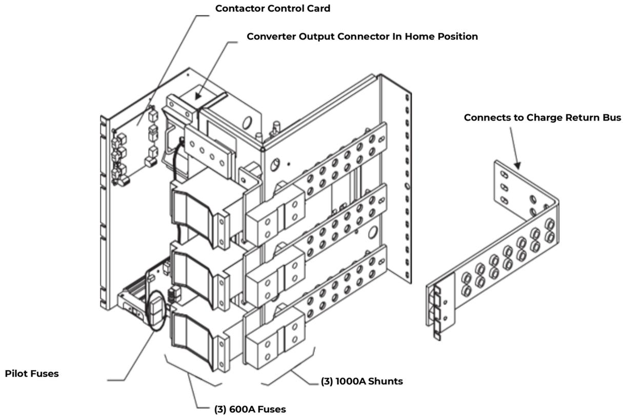
Figure 2-1: ED83143-30 Off Line Equalization (OLE) Panel
