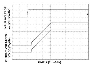
Figure 30. Typical Start-up Using Input Voltage (V<sub>IN</sub> = 12V, I<sub>o</sub> = I<sub>o1,max,</sub> I<sub>o2,max,</sub>).
