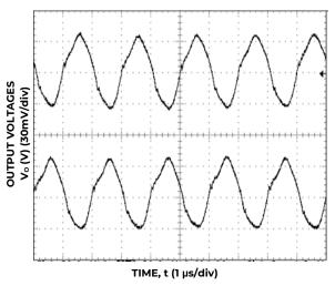
Figure 33. Typical output ripple and noise ( $C_0$ = 2×0.1uF+2×47uF ceramic,  $V_{IN}$  = 12V,  $I_0$  =  $I_{01,max,}I_{02,max,}$ ).
