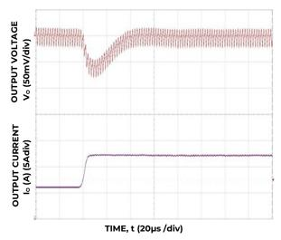
Figure 28 Transient Response to Dynamic Load Change on one output from 50% to 100% at 12Vin, Cout=3x47uF+1x330uF, CTune = 1200pF & RTune =  $300\Omega$
