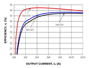
Figure 7. Converter Efficiency versus Output Current.
