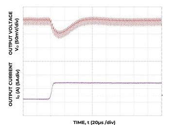
Figure 22. Transient Response to Dynamic Load Change from 50% to 100% on one output at 12 $V_{\rm in}$ ,  $C_{\rm out}$ =3x47uF+3x330uF,  $C_{\rm Tune}$ =1500pF &  $R_{\rm Tune}$ =300 $\Omega$
