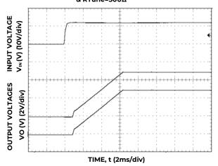
Figure 36. Typical Start-up Using Input Voltage  $(V_{IN} = 12V, I_o = I_{o1,max,} I_{o2,max,l})$ .
