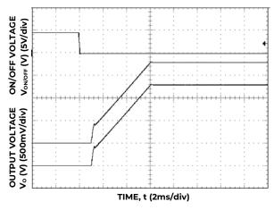
Figure 17. Typical Start-up Using On/Off Voltage ( $V_{IN}$ =12V,  $I_o$  =  $I_{Olymax, lo2,max,l}$ .
