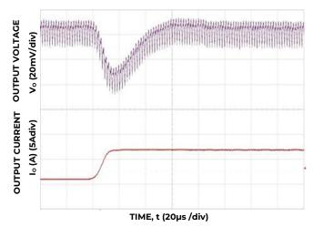
Figure 16. Transient Response to Dynamic Load Change from 50% to 100% on one output at 12V $_{in}$ , Cout=3x47uF+3x330uF, C $_{Tune}$ =1800pF &  $R_{Tune}$ =300 $\Omega$
