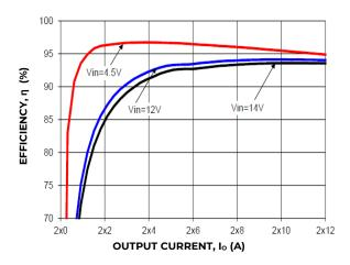
Figure 25. Converter Efficiency versus Output Current.
