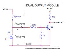
Figure 40. Circuit configuration for using negative On/Off logic.
