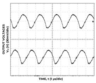
Figure 27. Typical output ripple and noise ( $C_0$ = 2×0.1uF+2×47uF ceramic,  $V_{IN}$  = 12V,  $I_0$  =  $I_{01,max}$ ,  $I_{02,max}$ , ).
