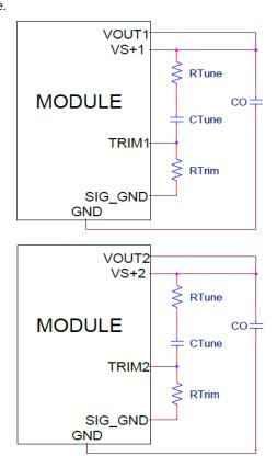
Figure. 47. Circuit diagram showing connection of  $R_{\text{TUNE}}$  and  $C_{\text{TUNE}}$  to tune the control loop of the module.
