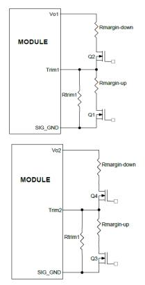
Figure 43. Circuit Configuration for margining Output voltage.
