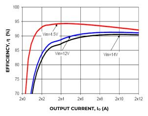
Figure 13. Converter Efficiency versus Output Current.
