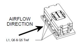
Figure 50. Preferred airflow direction and location of hotspot of the module (T<sub>ref</sub>).
