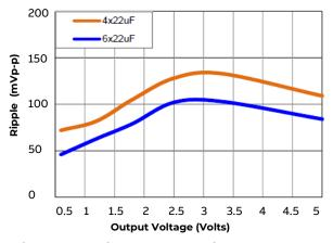
Figure 37. Input ripple voltage for various output voltages with 4x22  $\mu$ F or 6x22  $\mu$ F ceramic capacitors at the input (2 x 12A load). Input voltage is 12V
