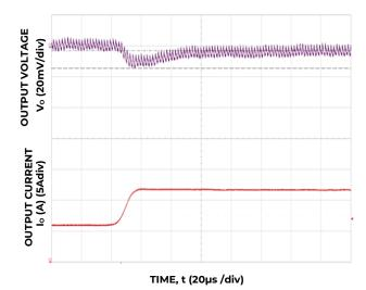
Figure 4. Transient Response to Dynamic Load Change from 50% to 100% on one output at 12V<sub>in</sub>, C<sub>out</sub>=2x47uF+7x330uF, C<sub>Tune</sub>=12nF. R<sub>Tune</sub>=300Ω
