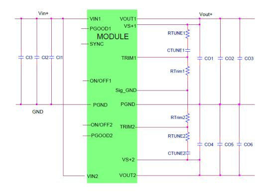
CII Decoupling cap - 4x0.1µF/16V, 0402 size ceramic capacitor
