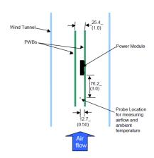
Figure 49. Thermal Test Setup.
