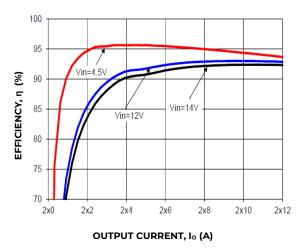
Figure 19. Converter Efficiency versus Output Current.
