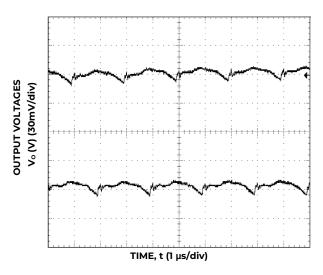
Figure 3. Typical output ripple and noise (Co=  $2\times0.1uF+2\times47uF$  ceramic,  $V_{IN}$  = 12V,  $I_o$  =  $I_{o1,max}$ ,  $I_{o2,max}$ ,).
