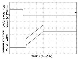
Figure 23. Typical Start-up Using On/Off Voltage  $(V_{IN}=12V, I_0 = I_{O1,max, I_{O2,max, i}})$ .
