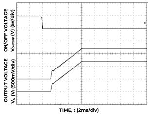
Figure 11. Typical Start-up Using On/Off Voltage ( $V_{IN}$ =12V,  $I_o$  =  $I_{o1,max,l}$ .
