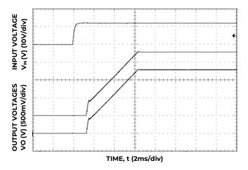
Figure 18. Typical Start-up Using Input Voltage ( $V_{IN}$  = 12V,  $I_0$  =  $I_{O1,max, I_{O2,max,i}}$ .
