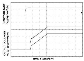
Figure 12. Typical Start-up Using Input Voltage ( $V_{IN}$  = 12V,  $I_o$  =  $I_{O1,max, Io2,max, I}$ .
