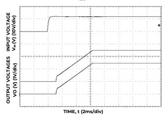
Figure 24. Typical Start-up Using Input Voltage ( $V_{IN}$  = 12V,  $I_0$  =  $I_{O1,max,l}$  |  $I_{O2,max,l}$ .
