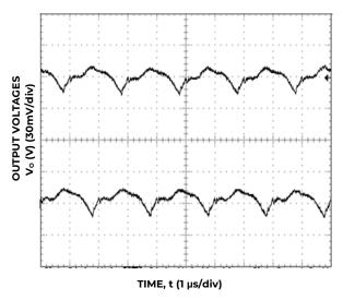
Figure 9. Typical output rippvle and noise ( $C_0$ = 2×0.1uF+2×47uF ceramic,  $V_{IN}$  = 12V,  $I_0$  =  $I_{01,max,}I_{02,max,}$ ).
