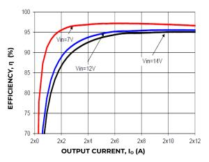
Figure 31. Converter Efficiency versus Output Current.
