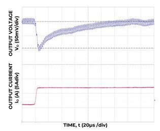
Figure 34. Transient Response to Dynamic Load Change on one output from 50% to 100% at 12Vin, Cout=6x47uF, CTune=470pF & RTune=300 $\Omega$
