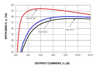
Figure 1. Converter Efficiency versus Output Current.
