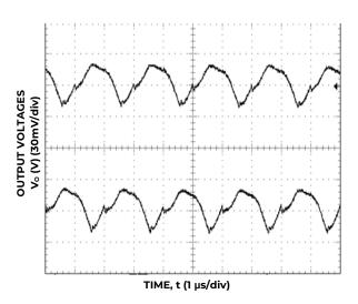
Figure 21. Typical output ripple and noise (Co= 2\*0.1uF+2\*47uF ceramic, V<sub>IN</sub> = 12V, Io = Io<sub>1,max</sub>, Io<sub>2,max</sub>,).
