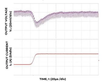
Figure 10. Transient Response to Dynamic Load Change from 50% to 100% on one output at  $12V_{in}$ ,  $C_{out}=3x47uF+3x330uF$ ,  $C_{Tune}=2700pF$  &  $R_{Tune}=300\Omega$
