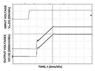
Figure 6. Typical Start-up Using Input Voltage ( $V_{IN}$  = 12V,  $I_o$  =  $I_{o_{I,max,i}}I_{o_{2,max,i}}$ .
