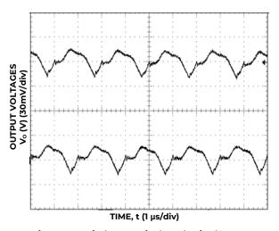
Figure 15. Typical output ripple and noise ( $C_0$ = 2×0.1uF+2×47uF ceramic,  $V_{IN}$  = 12V,  $I_0$  =  $I_{01,max}$ ,  $I_{02,max}$ ,  $I_{02}$
