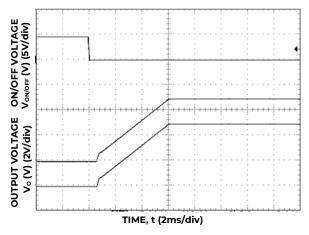
Figure 35. Typical Start-up Using On/Off Voltage  $(V_{IN}=12V, I_o=I_{o1,max}, I_{o2,max},)$ .
