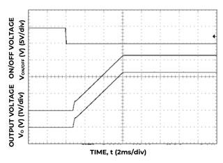
Figure 29. Typical Start-up Using On/Off Voltage (V<sub>IN</sub>=12V, I<sub>o</sub> = I<sub>Ol1max</sub>, I<sub>o2,max</sub>,).
