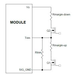
Figure 37. Circuit Configuration for margining Output voltage.
