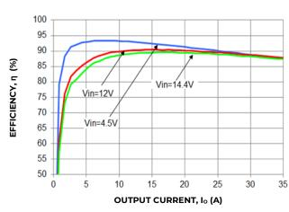
Figure 7. Converter Efficiency verses output current
