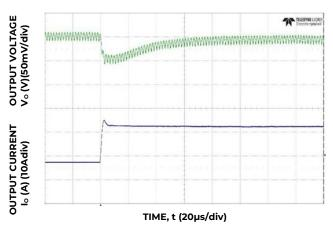
Figure 22. Transient Response to Dynamic Load Change on one output from 50% to 100% at 12V<sub>in</sub>, C<sub>out</sub> = 8x47uF + 4x330uF, C<sub>Tune</sub> = 3300pF & R<sub>Tune</sub> = 221Ω
