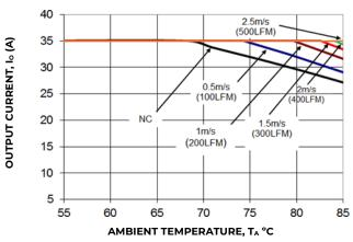
Figure 2. Derating Output Current verses Ambient Temperature and Airflow.
