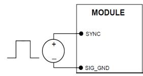
Figure 39. External source connections to synchronize switching frequency of the module.
