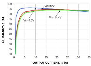
Figure 19. Converter Efficiency verses output current
