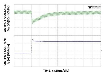
Figure 28. Transient Response to Dynamic Load Change on one output from 50% to 100% at 12V<sub>in</sub>, C<sub>out</sub> = 8x47uF + 2x330uF,
