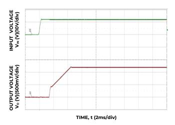
Figure 12. Typical Start-up Using Input Voltage (V<sub>IN</sub> = 12V, I₀ = I₀,max).
