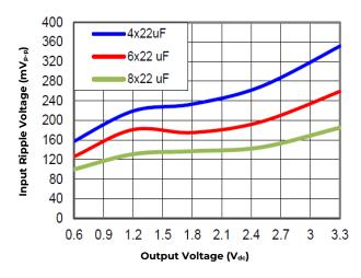
Figure 31. Input ripple voltage for various output voltages with 4x22  $\mu$ F, 6x22  $\mu$ F or 8x22  $\mu$ F ceramic capacitors at the input (35A load). Input voltage is 12V.
