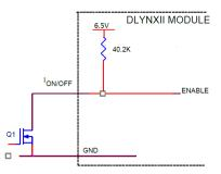
Figure 33. Circuit configuration for using positive On/Off logic.
