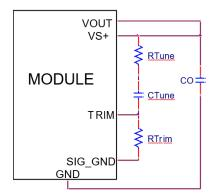
Figure. 40. Circuit diagram showing connection of  $R_{\text{TUNE}}$  and  $C_{\text{TUNE}}$  to tune the control loop of the module.
