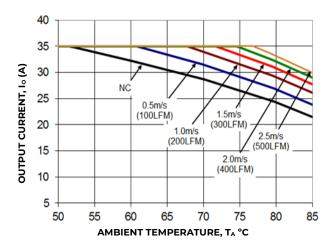
Figure 26. Derating Output Current verses Ambient Temperature and Airflow.
