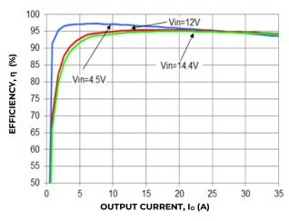
Figure 25. Converter Efficiency verses output current
