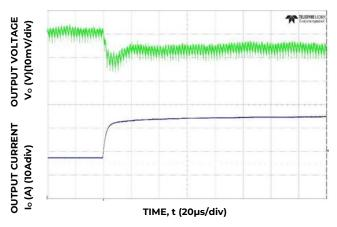
Figure 4. Transient Response to Dynamic Load Change from 50% to 100% at  $12V_{in}$ ,  $C_{out}$ =8x47uF+24x330uF,  $C_{Tune}$ =18nF,  $R_{Tune}$ =300 $\Omega$
