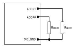
Figure 41. Circuit showing connection of resistors used to set the PMBus address of the module.
