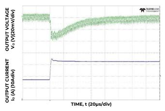
Figure 16. Transient Response to Dynamic Load Change on one output from 50% to 100% at 12V<sub>in</sub>, C<sub>out</sub> = 8x47uF + 7x330uF, C<sub>Tune</sub> = 4.7nF & R<sub>Tune</sub> = 221Ω
