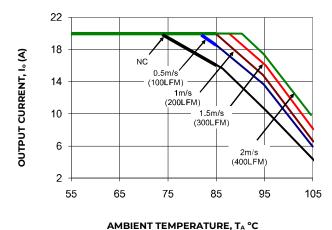
Figure 26. Derating Output Current versus Ambient
