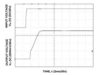
Figure 18. Typical Start-up Using Input Voltage ( $V_{\text{IN}}$  = 12V,  $I_{\text{o}}$  =  $I_{\text{o,max}}$ ).
