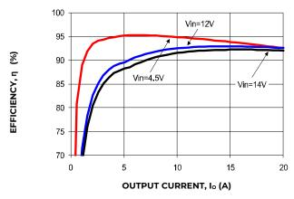
Figure 19 Converter Efficiency versus Output Current.
