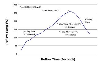
Figure 50. Recommended linear reflow profile using Sn/Ag/Cu
