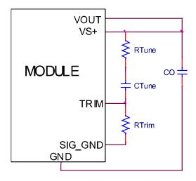
Figure. 46. Circuit diagram showing connection of  $R_{\text{TUNE}}$  and  $C_{\text{TUNE}}$  to tune the control loop of the module.
