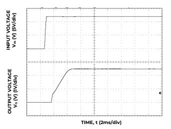
Figure 24. Typical Start-up Using Input Voltage  $(V_{\text{IN}}$  = 12V,  $I_{\text{o}}$  =  $I_{\text{o,max}}$ ).
