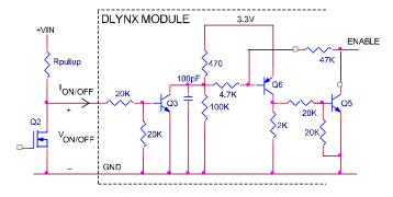
Figure 40. Circuit configuration for using negative On/Off logic.
