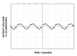
Figure 27. Typical output ripple and noise ( $C_0=2x47\mu F$  ceramic,  $V_{IN}=12V$ ,  $I_o=I_{o,max}$ ).
