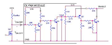
Figure 39. Circuit configuration for using positive On/Off logic.
