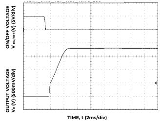
Figure 17. Typical Start-up Using On/Off Voltage (I<sub>o</sub> = I<sub>o,max</sub>).
