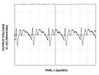
Figure 3. Typical output ripple and noise  $(C_0=2x47\mu F \text{ ceramic}, V_{IN}=12V, I_0=I_{0,max}).$
