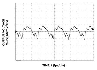
Figure 15. Typical output ripple and noise  $(C_0=2x47\mu F \text{ ceramic}, V_{IN}=12V, I_0=I_{o,max}).$
