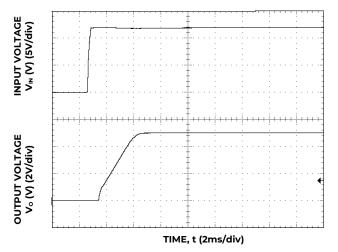
Figure 36. Typical Start-up Using Input Voltage  $(V_{IN} = 12V, I_0 = I_{0,max}).$
