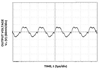
Figure 33. Typical output ripple and noise ( $C_0=2x47\mu F$  ceramic,  $V_{IN}=12V$ ,  $I_0=I_{o,max}$ ).
