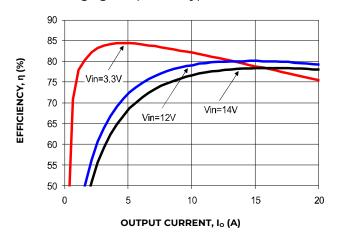
Figure 1. Converter Efficiency versus Output Current.
