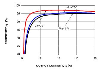
Figure 31. Converter Efficiency versus Output Current.
