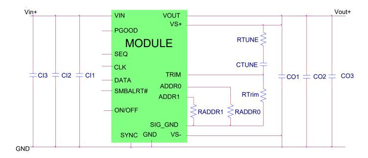
CII Decoupling cap - 1x0.047µF/16V ceramic capacitor (e.g. Murata LLL185R71C473MA01)
