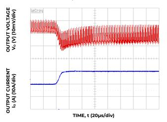
Figure 4. Transient Response to Dynamic Load Change from 50% to 100% at 12V $_{\rm in}$ , C $_{\rm out}$ = 1x47uF +11x330uF C $_{\rm Tune}$ =47nF, R $_{\rm Tune}$ =178 ohms
