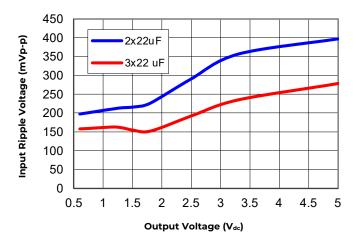
Figure 37. Input ripple voltage for various output voltages with 2x22  $\mu$ F or 3x22  $\mu$ F ceramic capacitors at the input (20A load). Input voltage is 12V.
