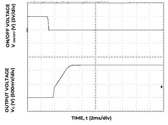
Figure 11. Typical Start-up Using On/Off Voltage ( $I_0 = I_{o,max}$ ).
