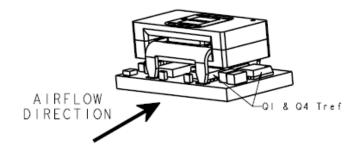
Figure 49. Preferred airflow direction and location of hotspot of the module ( $T_{\rm ref}$ ).
