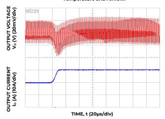
Figure 10. Transient Response to Dynamic Load Change from 50% to 100% at 12Vin, Cout= 1x47uF +5x330uF CTune=10nF, R<sub>Tune</sub>=178 ohms
