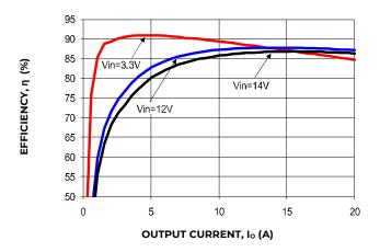
Figure 7. Converter Efficiency versus Output Current.
