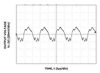
Figure 21. Typical output ripple and noise  $(C_0=2x47\mu F \text{ ceramic}, V_{IN}=12V, I_0=I_{o,max}).$
