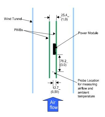
Figure 48. Thermal Test Setup.
