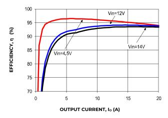
Figure 25 Converter Efficiency versus Output Current.
