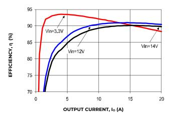
Figure 13 Converter Efficiency versus Output Current.
