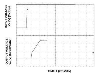
Figure 12. Typical Start-up Using Input Voltage
