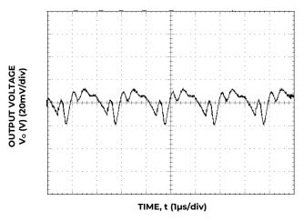
Figure 9. Typical output ripple and noise ( $C_0$ =2x47 $\mu$ F ceramic,  $V_{IN}$  = 12V,  $I_o$  =  $I_{o,max}$ ).
