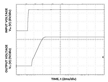
Figure 30. Typical Start-up Using Input Voltage ( $V_{\text{IN}}$  = 12V,  $I_{\text{o}}$  =  $I_{\text{o,max}}$ ).
