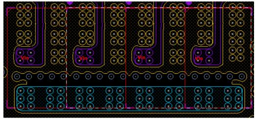
Figure 29. Example of Pad Layout with Vias
