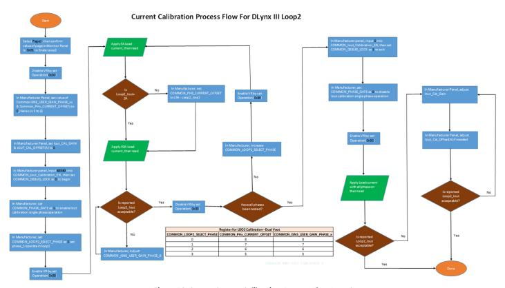
Figure 30. Output Current Calibration Process Flow-Loop 2
