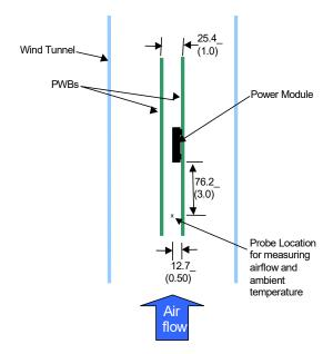
Figure 28. Thermal Test Setup.
