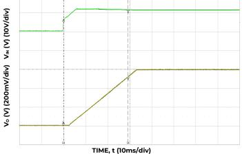
$_{\mbox{Page 4}}$  Figure 5. Typical Start-up Using On/Off Voltage (Io = Io, max).
