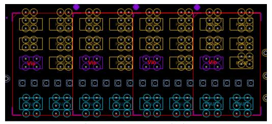
Figure 28. Example of Pad Layout with Vias
