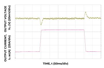
Figure 10. Trans. Resp. to 100A/µs Load Change from 25% to 75% at 12V<sub>IN</sub>, Co=4x0.047µF +4x0.1µF + 15x22µF + 73x47µF + 6x470µF polymer
