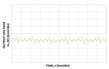
Figure 21. Typical output ripple ( $C_0$ =4x0.047 $\mu$ F +4x0.1 $\mu$ F + 15x22 $\mu$ F + 73x47 $\mu$ F + 6x470 $\mu$ F polymer,  $V_{IN}$  = 12V,  $I_0$  =  $I_{0,max}$ )
