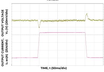
Figure 16. Trans. Resp. to 100A/ $\mu$ s Load Change from 25% to 75% at 12V $_{\text{IN}}$ , Co=4x0.047 $\mu$ F +4x0.1 $\mu$ F + 15x22 $\mu$ F + 73x47 $\mu$ F + 6x470 $\mu$ F polymer
