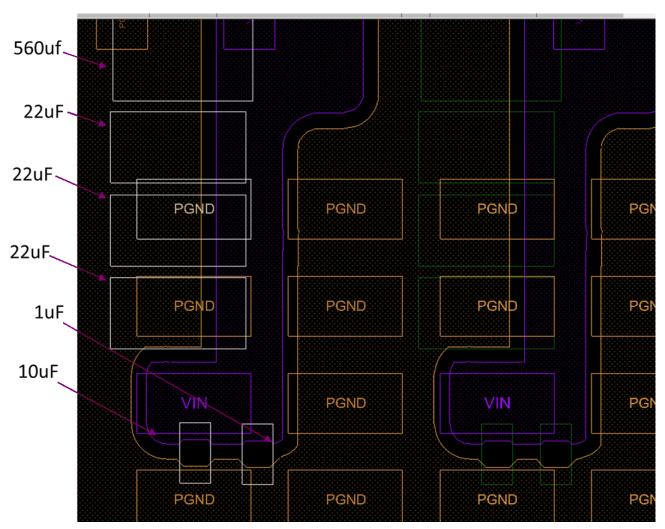
Figure 32. Input Capacitor Placement.
