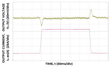
Figure 22. Trans. Resp. to 100A/μs Load Change from 25% to 75% at 12V<sub>IN</sub>, Co=4x0.047μF +4x0.1μF + 15x22μF + 73x47μF + 6x470μF polymer
