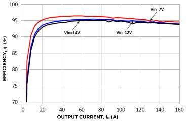
Figure 19. Converter Efficiency versus Output Current.
