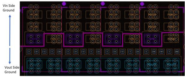
Figure 30. Example of split input-output ground
