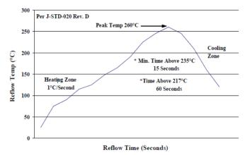
Figure 30. Recommended linear reflow profile using Sn/Ag/Cu solder
