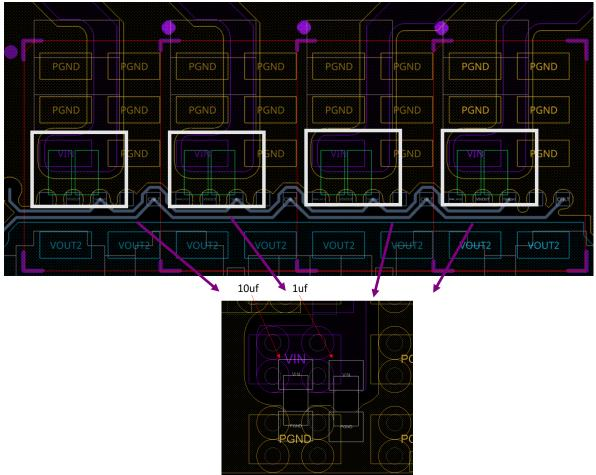
Figure 31. Example of Input capacitor placement and routing
