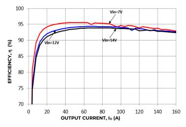
Figure 13. Converter Efficiency versus Output Current.
