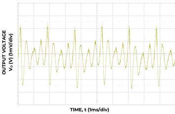
Figure 9. Typical output ripple( $C_0=4x0.047\mu F + 4x0.1\mu F + 15x22\mu F +$  $73x47\mu F + 6x470\mu F$  polymer,  $V_{IN} = 12V$ ,  $I_o = I_{o,max}$ ).
