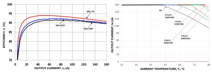
Figure 7. Converter Efficiency versus Output Current.
