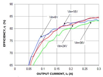
Figure 1. Converter Efficiency versus Output Current.
