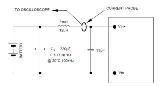
NOTE: Measure input reflected ripple current with a simulated source inductance ( $L_{\text{TEST}}$ ) of 12 $\mu$ H. Capacitor  $C_{\text{S}}$  offsets possible battery impedance. Measure current as shown above.
