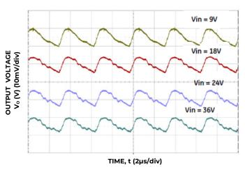
Figure 2. Typical output ripple and noise ( $V_o+$ ,  $I_o = I_{o,max}$ ).
