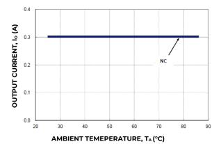
Figure 15. Output Current Derating for the Module with Heatplate; Airflow in the Transverse Direction from  $V_{out}(-)$  to  $V_{out}(+)$ ;  $V_{IN}$  =24V,  $V_{o}$ =+15V, -15V
