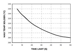
Figure 21. Time Limit, Tlim, Curve Above 205°C Reflow.
