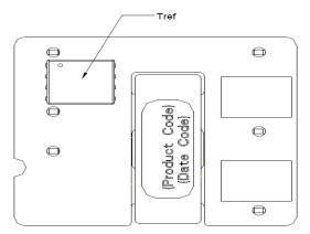
Figure 13. T<sub>ref</sub> Temperature Measurement Location.
