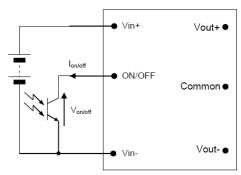
Figure 11. Circuit configuration for using Remote On/Off Implementation.
