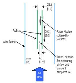
Figure 12. Thermal Test Setup.
