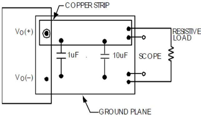
**Figure 8. Output Ripple and Noise Test Setup.**
