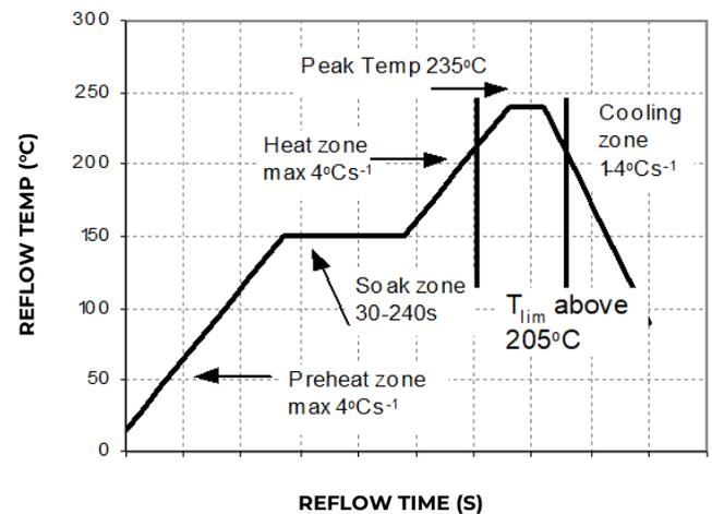
**Figure 20. Recommended Reflow Profile for Sn/Pb solder.**
