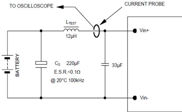
**Figure 7. Input Reflected Ripple Current Test Setup.**
