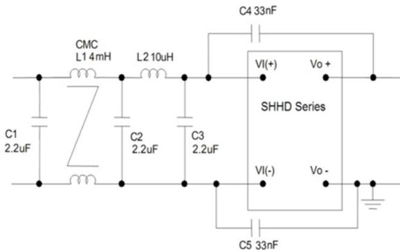
Figure 17. Suggested Configuration for EN55032 Class B.
