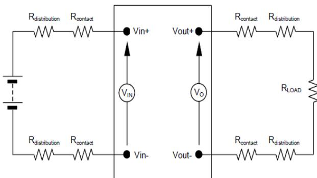
**Figure 9. Output Voltage and Efficiency Test Setup.**
