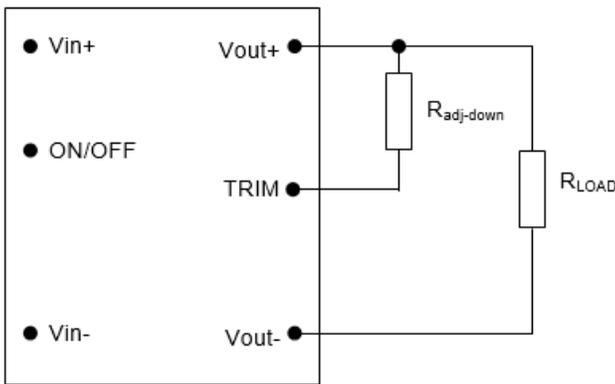
Figure 11. Circuit Configuration to Decrease Output Voltage.
