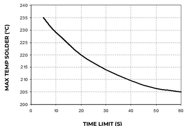
**Figure 21. Time Limit, T<sub>lim</sub>, Curve Above 205°C Reflow .**
