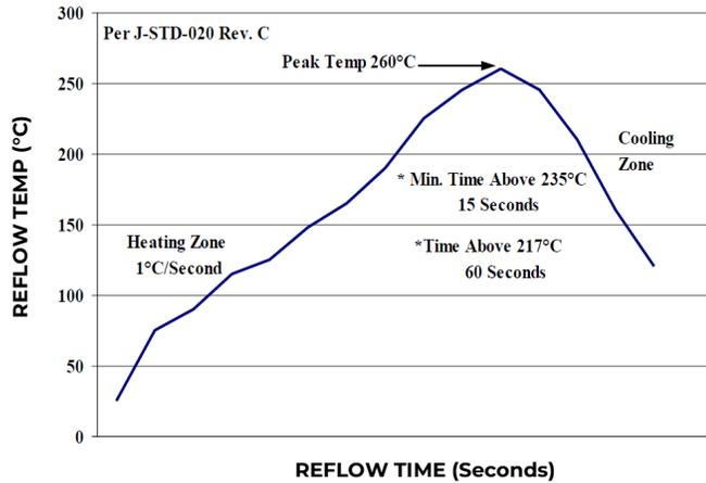
Figure 22. Recommended linear reflow profile using Sn/Ag/Cu solder
