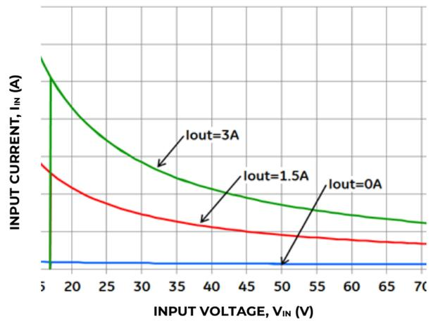
Figure 2. Converter Input Current versus Input Voltage.
