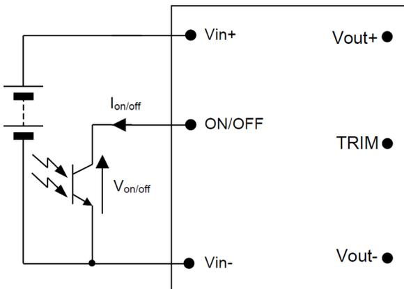
**Figure 10. Circuit configuration for using Remote On/Off Implementation.**
