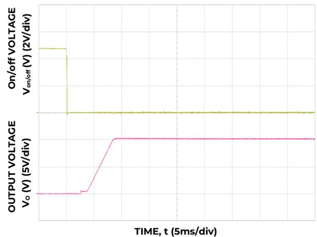
Figure 6. Typical Start-Up Using Remote On/Off with V<sub>in</sub> applied, negative logic version shown  $I_o = I_{o,max}$ .
