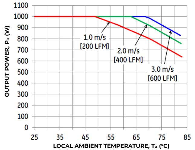
Figure 20. Output Power Derating with a 0.6" Heat Sink on QBVE094A0S10R7xx-H in the Longitudinal Orientation; Airflow Direction from V<sub>out</sub> to V<sub>in</sub>; V<sub>in</sub> = 51V.
