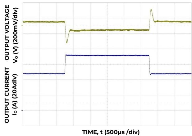
Figure 4. Typical Transient Response to 1A/μs Step Change in Load from 50% to 75% to 50% of Full Load,  $C_o = 3200\mu\text{f}$  and 48 V<sub>dc</sub> Input.
