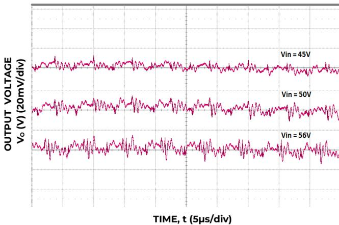
Figure 3. Typical output ripple and noise
