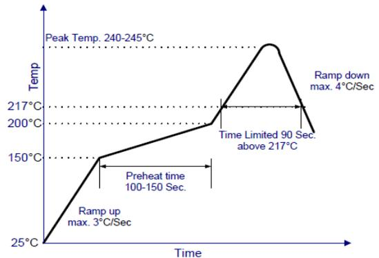
Figure 21. Recommended linear reflow profile using Sn/Ag/Cu solder
