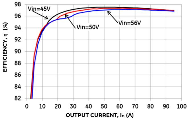
Figure 1. Typical Converter Efficiency versus Output Current.
