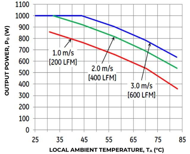
Figure 18. Output Power Derating for the Base Plate QBVE094A0S10R7xx-H in the Longitudinal Orientation; Airflow Direction from V<sub>out</sub> to V<sub>in</sub>; V<sub>in</sub> = 51V.
