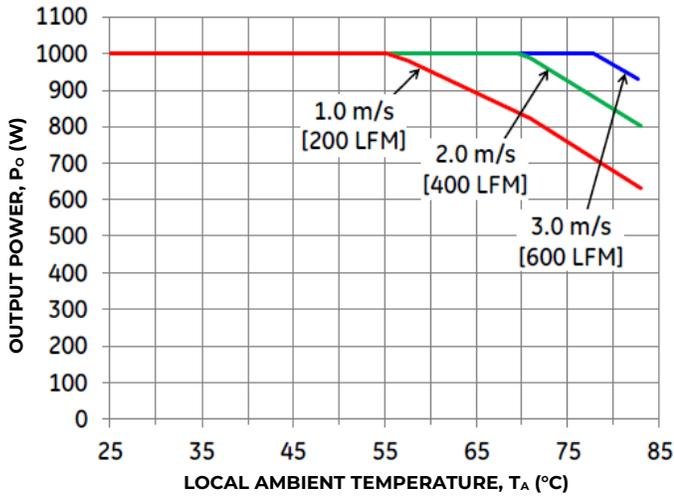
Figure 19. Output Power Derating with a 0.6" Heat Sink on QBVE094A0S10R7xx-H in the Transverse Orientation; Airflow Direction from V<sub>in</sub>(-) to V<sub>in</sub>(+); V<sub>in</sub> = 51V.
