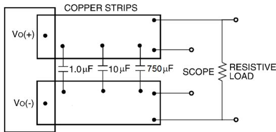
Note: Use a 1.0 μF ceramic capacitor, a 10 μF aluminum or tantalum capacitor and a 750μF polymer capacitor. Scope measurement should be made using a BNC socket. Position the load between 51 mm and 76 mm (2 in. and 3 in.) from the module.
