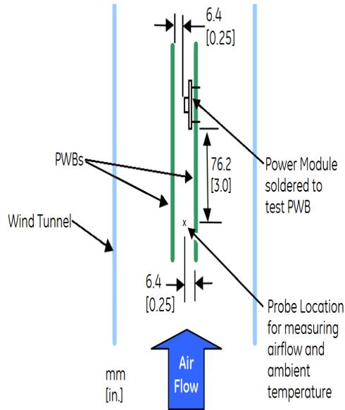
Figure 16. Thermal Test Setup .
