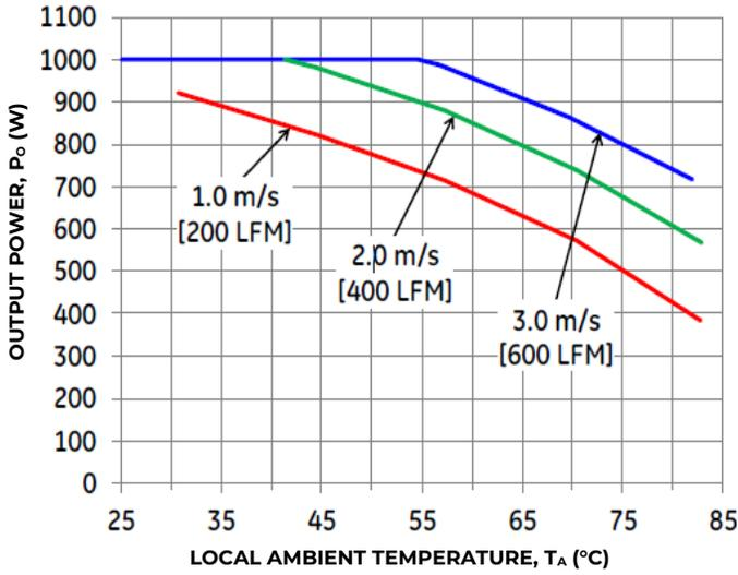
Figure 17. Output Power Derating for the Base plate QBVE094A0S10R7xx-H in the Transverse Orientation; Airflow Direction from V<sub>in</sub>(-) to V<sub>in</sub>(+); V<sub>in</sub> = 51V.
