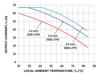
Figure 19. Output Current Derating for the Base Plate QBVE067A0Bxx-H in the Transverse Orientation; Airflow Direction from Vin(-) to Vin(+); Vin = 50V.
