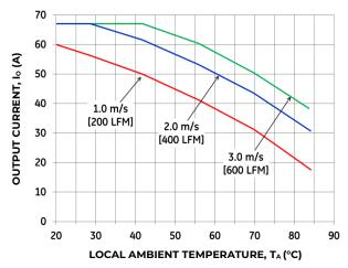
Figure 20. Output Current Derating for the Base plate QBVE067A0 Bxx-H in the Longitudinal Airflow Direction from Vout to Vin; Vin = 50V.
