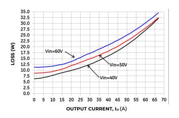
Figure 2. Typical Converter Loss vs. Output Current.
