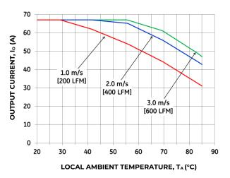
Figure 21. Output Current Derating for the Base plate QBVE067A0Bxx-H+0.5" Heat Sink in the Transverse Orientation; Airflow Direction from Vin(-) to Vin(+); Vin = 50V.
