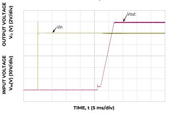
Figure 5. Typical Start-Up Using Vin with Remote On/Off enabled, negative logic version shown, I<sub>o</sub> = I<sub>oymax</sub>.
