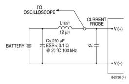
Figure 13. Input Reflected Ripple Current Test Setup.
