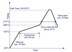
Figure 25. Recommended linear reflow profile using Sn/Ag/Cu solder.
