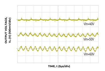
Figure 3. Typical Output Ripple and Noise,  $I_0 = I_{0,max} C_0 = 750 \mu F$ .
