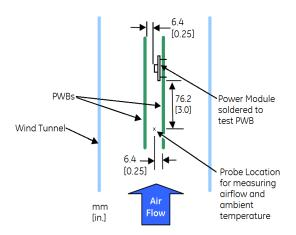
Figure 18. Thermal Test Setup .
