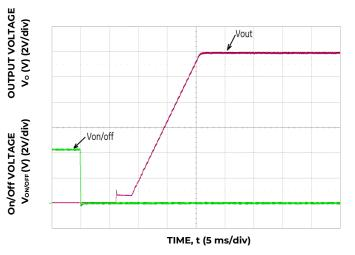
Figure 6. Typical Start-Up Using Remote On/Off with Vin applied, negative logic version shown I<sub>o</sub> = I<sub>o,max</sub>.
