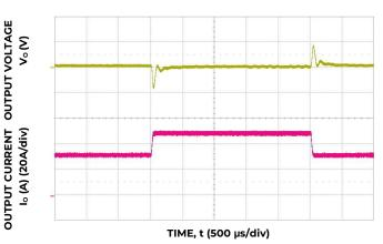
Figure 4. Typical Transient Response to 1.0A/ $\mu$ s Step Change in Load from 50% to 75% to 50% of Full Load, C<sub>o</sub>=470 $\mu$ F and 50 V<sub>dc</sub> Input.
