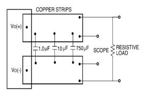
Figure 14. Output Ripple and Noise Test Setup.
