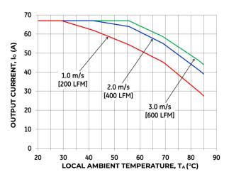
Figure 22. Output Current Derating for the Base plate QBVE067A0Bxx-H+0.5" Heat Sink in the Longitudinal Airflow Direction from Vout to Vin; Vin = 50V.
