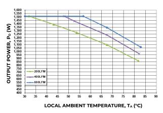
Figure 21. Output Power Derating for the Integrated Heatsink version QBDS128A0B-F; Airflow Direction for Vin- to Vin+ orientation; Vin = 50V.
