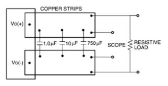
Note: Use a 1.0  $\mu$ F ceramic capacitor, a 10  $\mu$ F aluminum or tantalum capacitor and a 750 polymer capacitor. Scope measurement should be made using a BNC socket. Position the load between 51 mm and 76 mm (2 in. and 3 in.) from the module.
