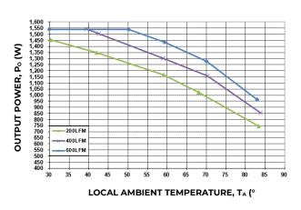
Figure 20. Output Power Derating for the Base plate QBDS128A0B1-H+0.44" Heat Sink; Airflow Direction for Vout to Vin(Worst) orientation; Vin = 54V.
