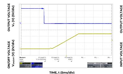
Figure 5. Typical Start-up Using On/Off Voltage (Io = Io,max).
