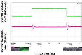
Figure 4. Dynamic Load Response, dI<sub>0</sub>/dt=1A/us; V<sub>in</sub>=V<sub>in,nom</sub>; T<sub>A</sub>=25°C; Load Change from I<sub>0</sub> = 50% to 75% of I<sub>0,max</sub>; C<sub>0</sub> =6160µF Ceramic;
