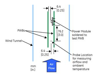
Figure 23. Thermal Test Setup
