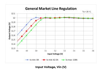
Figure 9. Typical Output Voltage Regulation vs Input Voltage, without droop
