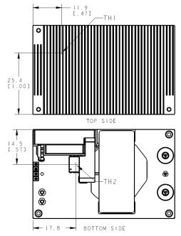
Figure 16. Location of the thermal reference temperature TH1 and TH2 for integrated heatsink module.
