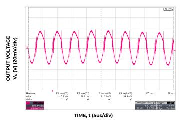
Figure 3. Typical output ripple and noise ( $C_o$  = 650 $\mu$ F Ceramic + 650 $\mu$ F PosCap Oscon ,  $V_{in}$  = 54V,  $I_o$  =  $I_{o,max}$ , ).
