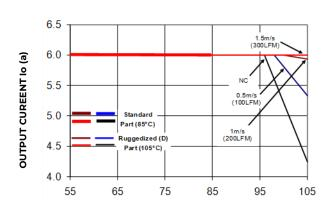
AMBIENT TEMPERATURE, T<sub>A</sub> °C Figure 26 Derating Output Current versus Ambient Temperature and Airflow.
