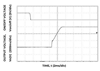
Figure 5. Typical Start-up Using On/Off Voltage (I<sub>o</sub> = I<sub>o</sub>,max).
