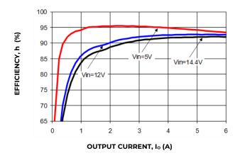
Figure 25. Converter Efficiency versus Output Current.
