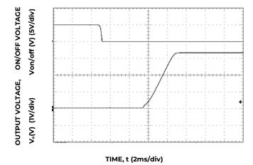
Figure 29. Typical Start-up Using On/Off Voltage (I<sub>o</sub> = I<sub>o</sub>,max).
