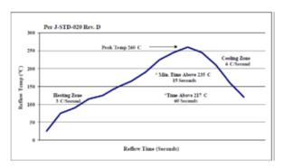
Figure 48. Recommended linear reflow profile using Sn/Ag/Cu solder.
