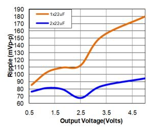
Figure 38. Input ripple voltage for various output voltages with 1x22 µF or 2x22 µF ceramic capacitors at the input (6A load). Input voltage is 12V.
