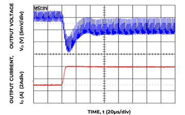
Figure 4. Transient Response to Dynamic Load Change from 50% to 100% at 9Vin, Cout-2x47uF+4x330uF, CTune-33nF, RTune-178
