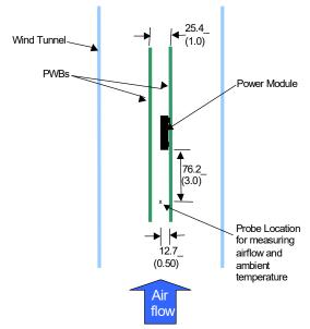
Figure 47. Thermal Test Setup.
