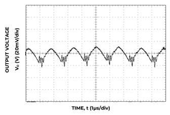
Figure 9. Typical output ripple and noise ( $C_0=10\mu F$  ceramic,  $V_{IN}=12V,\ I_o=I_{o,max}$ ,).
