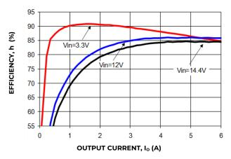
Figure 7. Converter Efficiency versus Output Current.
