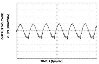
Figure 21. Typical output ripple and noise ( $C_0=10\mu F$  ceramic,  $V_{IN}=12V,\ I_o=I_{o,max}$ ,).
