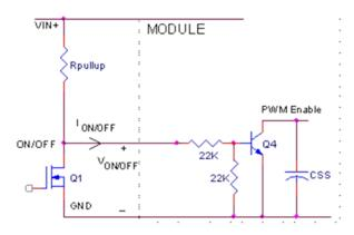
Figure 41. Circuit configuration for using negative On/Off logic.
