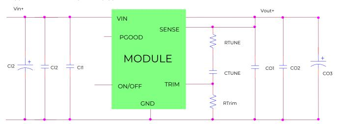
CII Decoupling cap - 1x0.047uF/16V ceramic capacitor (e.g. Murata LLL185R71C473MA01)
