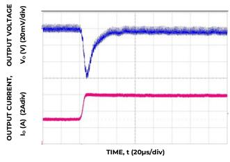
Figure 22. Transient Response to Dynamic Load Change from 50% to 100% at 12Vin, Cout-3x47uF, CTune-3300nF, RTune-178
