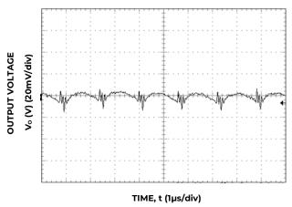
Figure 3. Typical output ripple and noise (Co=10 $\mu$ F ceramic, V<sub>IN</sub> = 8V, Io = Io, max, ).
