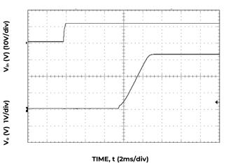
Figure 30. Typical Start-up Using Input Voltage ( $V_{IN}$  = 12V,  $I_0$  =  $I_0$ , max).
