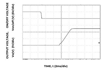
Figure 23. Typical Start-up Using On/Off Voltage (I<sub>o</sub> = I<sub>o</sub>,max).
