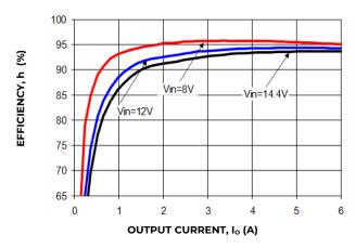
Figure 31. Converter Efficiency versus Output Current.
