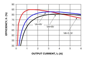
Figure 1. Converter Efficiency versus Output Current.
