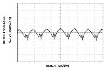
Figure 15. Typical output ripple and noise (Co=10µF ceramic,  $V_{\text{IN}}$  = 12V,  $I_{\text{o}}$  =  $I_{\text{o}}$ ,max, ).
