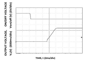
Figure 17. Typical Start-up Using On/Off Voltage (I<sub>o</sub> = I<sub>o</sub>,max).
