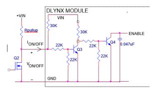
Figure 40. Circuit configuration for using positive On/Off logic.
