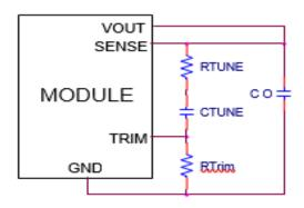
Figure. 46. Circuit diagram showing connection of  $R_{\text{TUME}}$  and  $C_{\text{TUNE}}$  to tune the control loop of the module.
