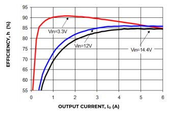
Figure 13. Converter Efficiency versus Output Current.
