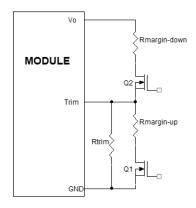
Figure 44. Circuit Configuration for margining Output voltage.
