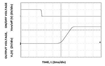
Figure 35. Typical Start-up Using On/Off Voltage (I<sub>o</sub> = I<sub>o</sub>,max).
