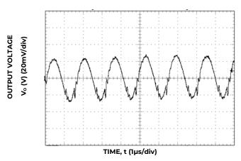
Figure 27. Typical output ripple and noise ( $C_0$ =10 $\mu$ F ceramic, VIN = 12V,  $I_o$  =  $I_o$ ,max, ).
