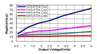
Figure 39. Output ripple voltage for various output voltages with external Ix10uF, 1x22uF, 1x47uF and 2x47uF ceramic capacitors at the output (6A load). Input voltage is 12V.
