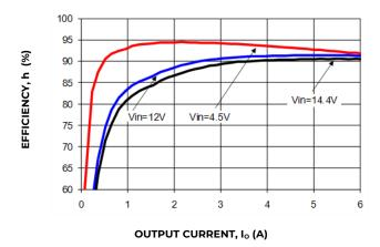
Figure 19. Converter Efficiency versus Output Current.
