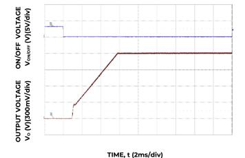
Figure 11. Typical Start-up Using On/Off Voltage  $(I_0 = I_{0,max})$ .
