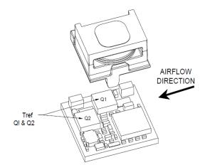
Figure 42. Preferred airflow direction and location of hot-spot of the module  $(T_{\rm ref})$ .
