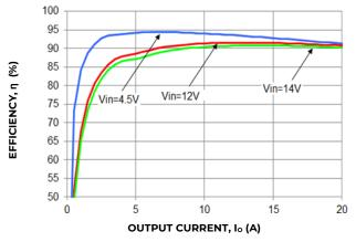
Figure 13. Converter Efficiency verses output current
