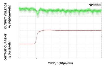
Figure 4. Transient Response to Dynamic Load Change from 50% to 100% at 12Vin,  $C_{\text{out}}$ = 7x47 $\mu$ F + 9x330 $\mu$ F,  $C_{\text{Tune}}$ =15nF,  $R_{\text{Tune}}$ =300
