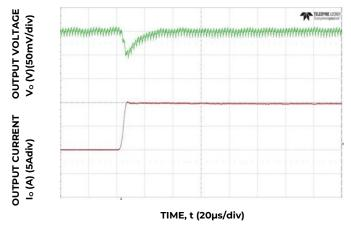
Figure 22. Transient Response to Dynamic Load Change from 50% to 100% at 12 $V_{in}$ ,  $C_{out}$ = 7x47 $\mu$ F+1x330 $\mu$ F,  $C_{Tune}$ =2700pF,  $R_{Tune}$ =300
