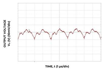
Figure 9. Typical output ripple ( $C_0=7x22 \mu F$  ceramic,  $V_{IN}=12V$ ,  $I_0=I_{o,max}$ ).
