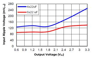
Figure 31. Input ripple voltage for various output voltages with 4x22  $\mu F$  or 6x22  $\mu F$  ceramic capacitors at the input (20A load). Input voltage is 12V.
