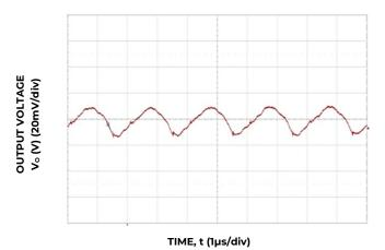
Figure 27. Typical output ripple and noise (Co=7x22µF ceramic, V<sub>IN</sub> = 12V, I<sub>o</sub> = I<sub>o,max,</sub>).
