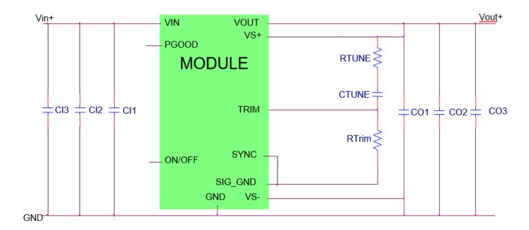
CII Decoupling cap - 1x0.047µF/16V ceramic(e.g. Murata LLL185R71C473MA01) + 1x0.1µF/16V 0402 ceramic
