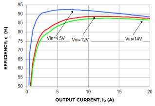
Figure 7. Converter Efficiency verses output current
