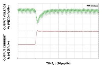
Figure 16. Transient Response to Dynamic Load Change from 50% to 100% at 12V<sub>in</sub>, C<sub>out</sub>= 7x47μF + 2x330μF, C<sub>Tune</sub>=3900pF
