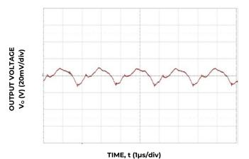
Figure 21. Typical output ripple and noise  $(C_0=7x22\mu F \text{ ceramic}, V_{IN}=12V, I_0=I_{0,max})$ .
