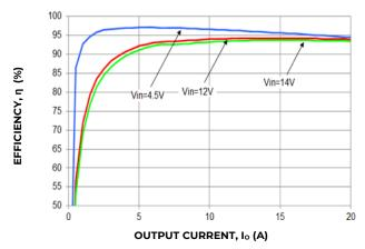
Figure 25. Converter Efficiency verses output current
