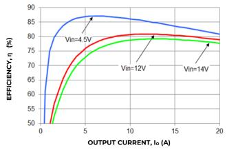
Figure 1. Converter Efficiency verses output current
