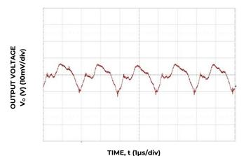
Figure 15. Typical output ripple (C<sub>0</sub>=7x22 $\mu$ F ceramic, V<sub>IN</sub> = 12V, I<sub>0</sub> = I<sub>0,max</sub>,).
