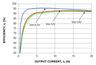
Figure 19. Converter Efficiency verses output current
