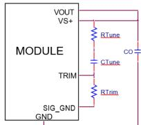
Figure. 40. Circuit diagram showing connection of  $R_{\text{TUME}}$  and  $C_{\text{TUNE}}$  to tune the control loop of the module.
