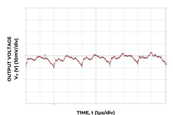
Figure 3. Typical output ripple (Co=7x22µF ceramic, V<sub>IN</sub> = 12V, I<sub>o</sub> = I<sub>o,max</sub>,).
