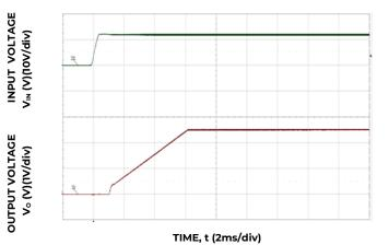
Figure 24. Typical Start-up Using Input Voltage  $(V_{\text{IN}}=12V,\,I_o=I_{o,\text{max}}).$
