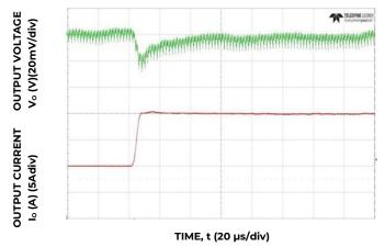
Figure 10. Transient Response to Dynamic Load Change from 50% to 100% at 12V $_{in}$ ,  $C_{out}$ = 7x47 $\mu$ F + 4x330  $\mu$ F,  $C_{Tune}$ =6800 $\rho$ F,  $R_{Tune}$ =300
