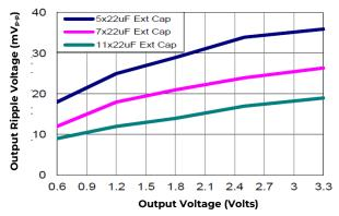
Figure 38. Output ripple voltage for various output voltages with external 5x22  $\mu$ F, 7x22  $\mu$ F or 11x22  $\mu$ F ceramic capacitors at the output (20A load). Input voltage is 12V.
