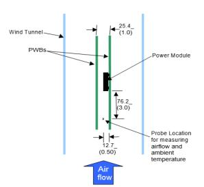
Figure 41. Thermal Test Setup.
