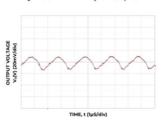
Figure 27. Typical output ripple ( $C_0$ =7x22 $\mu$ F ceramic,  $V_{IN}$  = 12V, Io =  $I_{o,max,}$ ).
