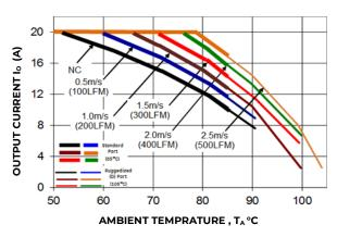
Figure 26. Derating Output Current versus
