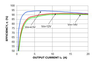
Figure 13. Converter Efficiency versus Output Current.
