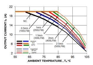
Figure 14. Derating Output Current versus
