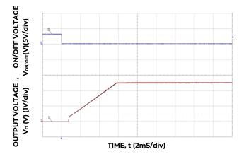
Figure 23. Typical Start-up Using On/Off Voltage (Io = I<sub>o,max</sub>).
