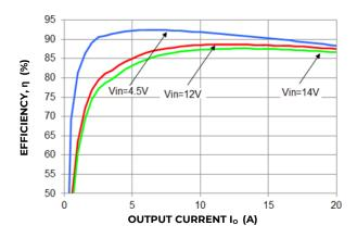
Figure 7. Converter Efficiency versus Output Current.
