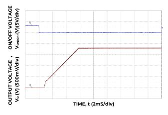
Figure 17. Typical Start-up Using On/Off Voltage (Io = I<sub>o,max</sub>).
