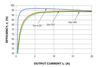
Figure 25. Converter Efficiency versus Output Current.
