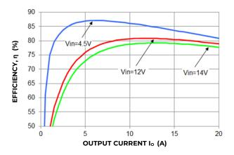
Figure 1. Converter Efficiency versus Output Current.
