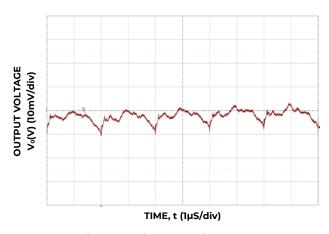
Figure 3. Typical output ripple (C₀=7x22µF ceramic,  $V_{IN}$  = 12V, Io =  $I_{o,max}$ ,).
