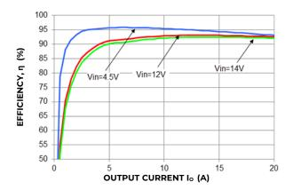
Figure 19. Converter Efficiency versus Output Current.
