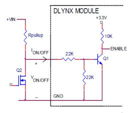
Figure 40. Circuit configuration for using negative On/Off logic.
