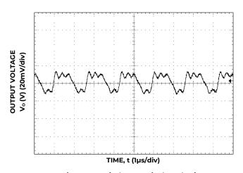
Figure 15. Typical output ripple and noise ( $C_0$ =22 $\mu$ F ceramic,  $V_{IN}$  = 12V,  $I_0$  =  $I_{o,max_1}$ ).
