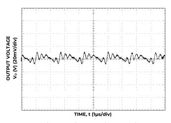
Figure 9. Typical output ripple and noise ( $C_0=22\mu F$  ceramic,  $V_{IN}=12V$ ,  $I_0=I_{0,max}$ ).
