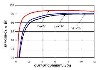
Figure 31. Converter Efficiency versus output current
