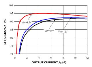
Figure 19. Converter Efficiency versus output current
