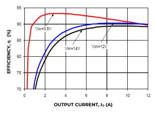
Figure 13. Converter Efficiency versus output current
