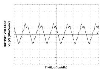
Figure 33. Typical output ripple and noise ( $C_0$ =22 $\mu$ F ceramic,  $V_{IN}$  = 12V,  $I_o$  =  $I_{o,max}$ ,).
