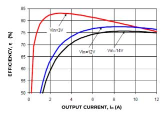
Figure 1. Converter Efficiency versus output current
