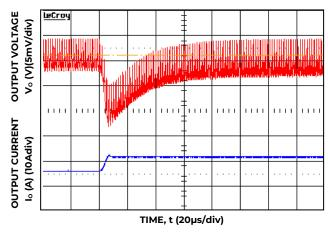
Figure 4. Transient Response to Dynamic Load Change from 50% to 100% at 12V<sub>in</sub>, C<sub>out</sub>=3x47uF+6x330uF, C<sub>Tune</sub>=47nF, R<sub>Tune</sub>=1800hm
