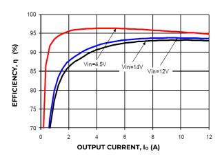
Figure 25. Converter Efficiency versus output current
