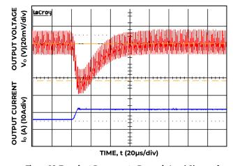
Figure 16. Transient Response to Dynamic Load Change from 50% to 100% at 12 $V_{in}$ ,  $C_{out}$ =1x4 $T_{uF}$ +2x330uF,  $C_{Tune}$ =5600pF,  $R_{Tune}$ =2700hms
