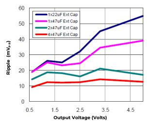
Figure 38. Output ripple voltage for various output voltages with external 1x22 μF, 1x47 μF, or 4x47 μF ceramic capacitors at the output (12A load). Input voltage is 12V.
