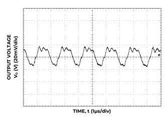
Figure 21. Typical output ripple and noise  $(C_0=22\mu F \text{ ceramic}, V_{IN}=12V, I_0=I_{o,max,}).$
