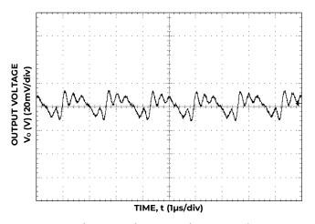
Figure 3. Typical output ripple and noise ( $C_0$ =22 $\mu$ F ceramic,  $V_{IN}$  = 12V,  $I_o$  =  $I_{o,max_0}$ ).
