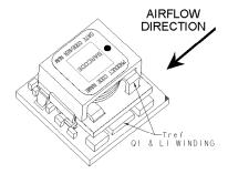
Figure 50. Preferred airflow direction and location of hot-spot of the module ( $T_{\rm ref}$ ).
