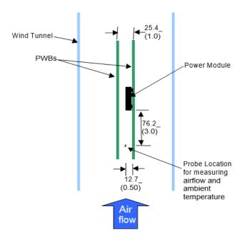
Figure 49. Thermal Test Setup.
