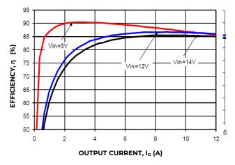
Figure 7. Converter Efficiency versus output current
