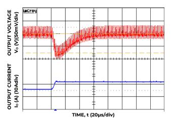
Figure 28. Transient Response to Dynamic Load Change from 50% to 100% at 12 $V_{in}$ ,  $C_{out}$ =1x47uF+ 1x330uF,  $C_{Tune}$ =2700pF, R<sub>Tune</sub>=330ohms
