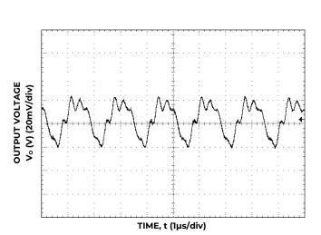
Figure 27. Typical output ripple and noise (C<sub>0</sub>=22 $\mu$ F ceramic, V<sub>IN</sub> = 12V, I<sub>0</sub> = I<sub>0,max</sub>,).
