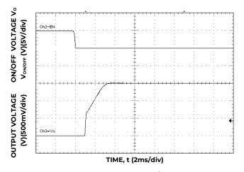
Figure 11. Typical Start-up Using On/Off Voltage (I $_{\rm o}$  = I $_{\rm o,max}$ ).
