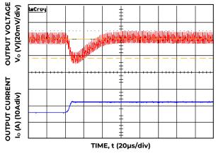
Figure 22. Transient Response to Dynamic Load Change from 50% to 100% at 12 $V_{in}$ ,  $C_{out}$ =1x47uF+ 1x33uF,  $C_{Tune}$ =3300pF,  $R_{Tune}$ =270 ohms
