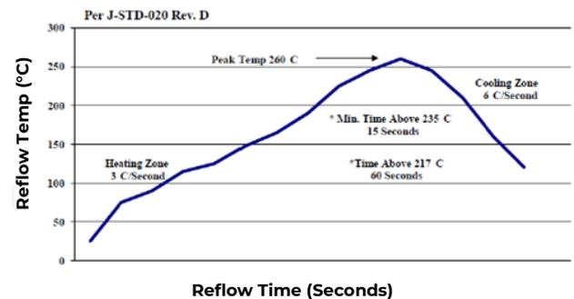
Figure 51. Recommended linear reflow profile using Sn/Ag/Cu solder.
