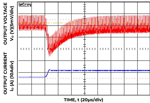
Figure 4. Transient Response to Dynamic Load Change from 50% to 100% at 12V<sub>in</sub>, C<sub>out</sub>=3x47μF+6x330μF, C<sub>Tune</sub>=47nF, R<sub>Tune</sub>=180ohm.
