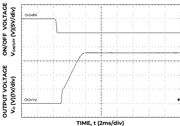
Figure 23. Typical Start-up Using On/Off Voltage (I<sub>o</sub> = I<sub>o,max</sub>).
