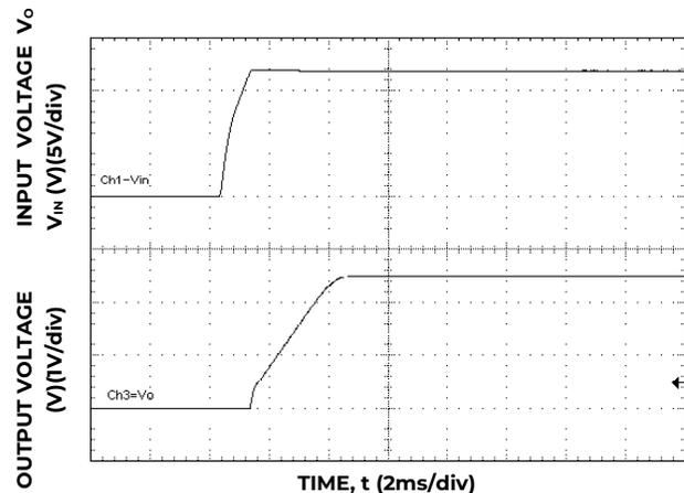
Figure 24. Typical Start-up Using Input Voltage (V<sub>IN</sub> = 12V, I<sub>o</sub> = I<sub>o,max</sub>).
