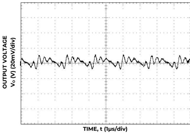
Figure 9. Typical output ripple and noise (C<sub>o</sub>=22μF ceramic, V<sub>IN</sub> = 12V, I<sub>o</sub> = I<sub>o,max</sub>).
