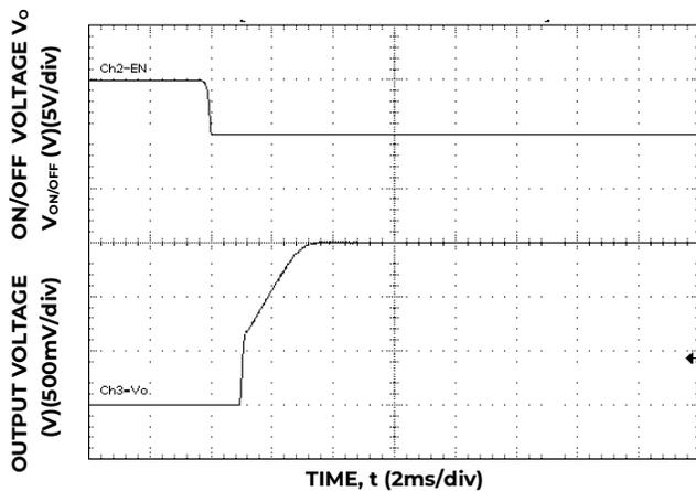
Figure 11. Typical Start-up Using On/Off Voltage (I<sub>o</sub> = I<sub>o,max</sub>).
