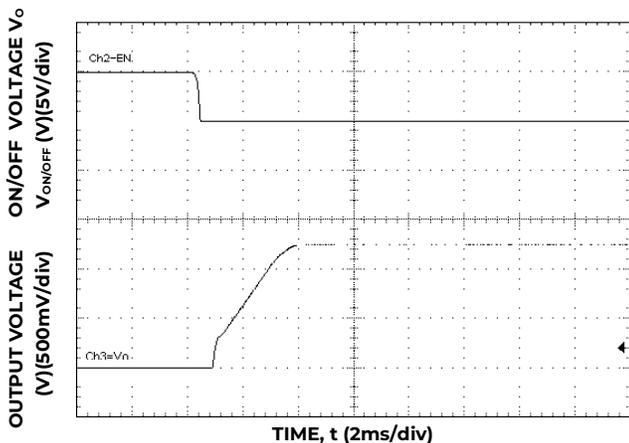
Figure 17. Typical Start-up Using On/Off Voltage (I<sub>o</sub> = I<sub>o,max</sub>).
