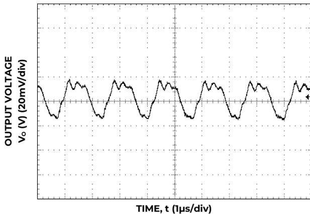
Figure 21. Typical output ripple and noise (C<sub>o</sub>=22μF ceramic, V<sub>IN</sub> = 12V, I<sub>o</sub> = I<sub>o,max</sub>).
