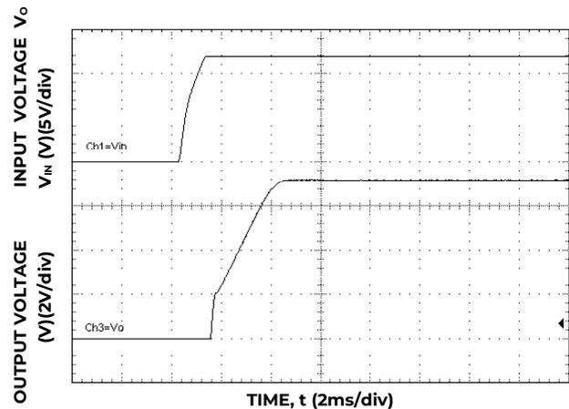
Figure 36. Typical Start-up Using Input Voltage (V<sub>IN</sub> = 12V, I<sub>o</sub> = I<sub>o,max</sub>).
