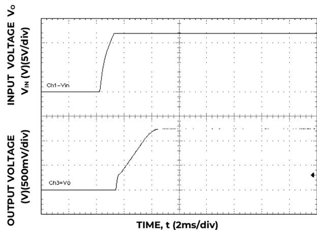
Figure 18. Typical Start-up Using Input Voltage (V<sub>IN</sub> = 12V, I<sub>o</sub> = I<sub>o,max</sub>).
