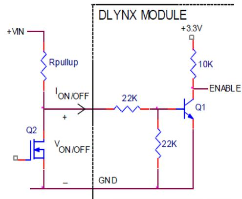
Figure 40. Circuit configuration for using negative On/Off logic.
