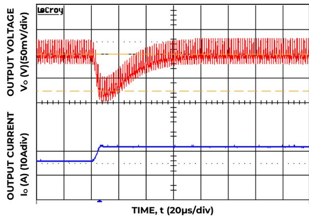
Figure 28. Transient Response to Dynamic Load Change from 50% to 100% at 12V<sub>in</sub>, C<sub>out</sub>=1x47μF+ 1x330μF, C<sub>Tune</sub>=2700pF, R<sub>Tune</sub>=330ohms.
