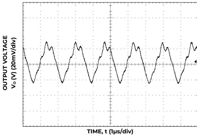
Figure 33. Typical output ripple and noise (C<sub>o</sub>=22μF ceramic, V<sub>IN</sub> = 12V, I<sub>o</sub> = I<sub>o,max</sub>).
