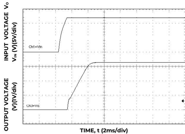
Figure 30. Typical Start-up Using Input Voltage (V<sub>IN</sub> = 12V, I<sub>o</sub> = I<sub>o,max</sub>).
