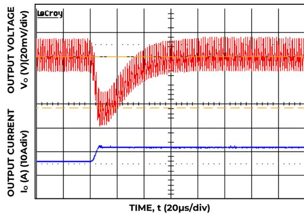
Figure 16. Transient Response to Dynamic Load Change from 50% to 100% at 12V<sub>in</sub>, C<sub>out</sub>=1x47μF+2x330μF, C<sub>Tune</sub>=5600pF, R<sub>Tune</sub>=270ohms.
