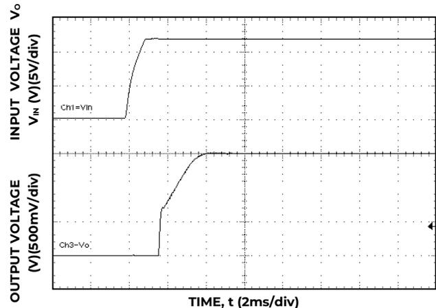
Figure 12 Typical Start-up Using Input Voltage (V<sub>IN</sub> = 12V, I<sub>o</sub> = I<sub>o,max</sub>).
