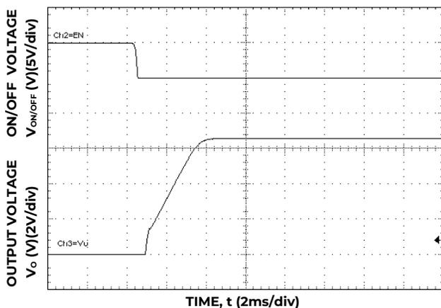
Figure 35. Typical Start-up Using On/Off Voltage (I<sub>o</sub> = I<sub>o,max</sub>).
