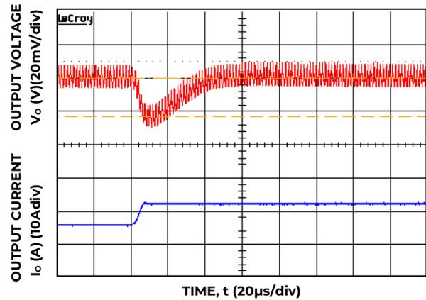
Figure 22. Transient Response to Dynamic Load Change from 50% to 100% at 12V<sub>in</sub>, C<sub>out</sub>=1x47μF+ 1x33μF, C<sub>Tune</sub>=3300pF, R<sub>Tune</sub>=270 ohms.
