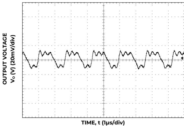
Figure 15. Typical output ripple and noise (C<sub>o</sub>=22μF ceramic, V<sub>IN</sub> = 12V, I<sub>o</sub> = I<sub>o,max</sub>).
