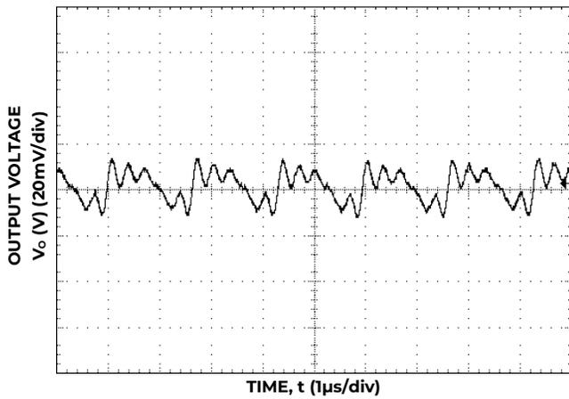
Figure 3. Typical output ripple and noise (C<sub>o</sub>=22μF ceramic, V<sub>IN</sub> = 12V, I<sub>o</sub> = I<sub>o,max</sub>).
