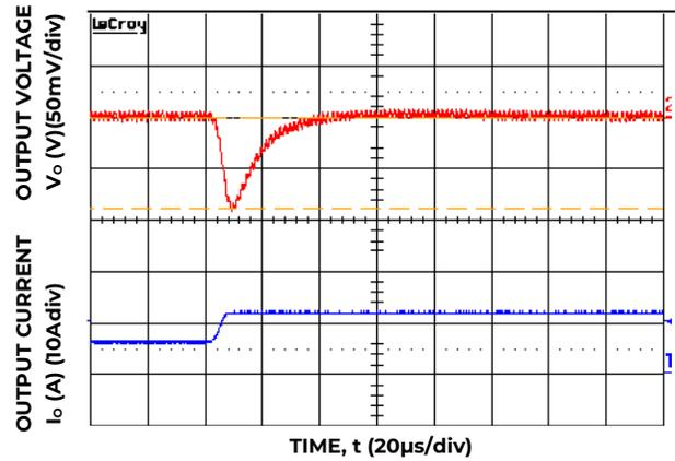
Figure 34. Transient Response to Dynamic Load Change from 50% to 100% at 12V<sub>in</sub>, C<sub>out</sub>=5x47μF, C<sub>Tune</sub>=1500pF, R<sub>Tune</sub>=330 ohms.
