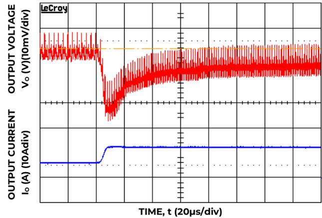
Figure 10. Transient Response to Dynamic Load Change from 50% to 100% at 12V<sub>in</sub>, C<sub>out</sub>=1x47μF+3x330μF, C<sub>Tune</sub>=10nF, R<sub>Tune</sub>=220ohms
