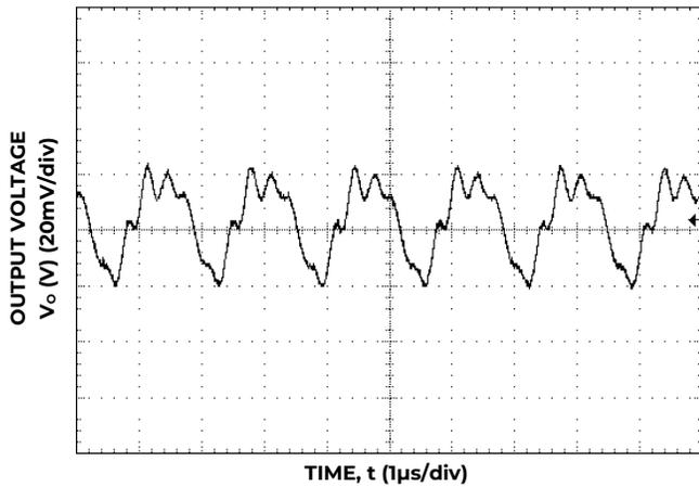
Figure 27. Typical output ripple and noise (C<sub>o</sub>=22μF ceramic, V<sub>IN</sub> = 12V, I<sub>o</sub> = I<sub>o,max</sub>).
