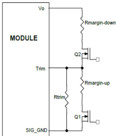
Figure 43. Circuit Configuration for margining Output voltage.
