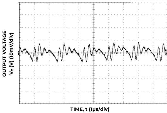
Figure 3. Typical output ripple and noise
