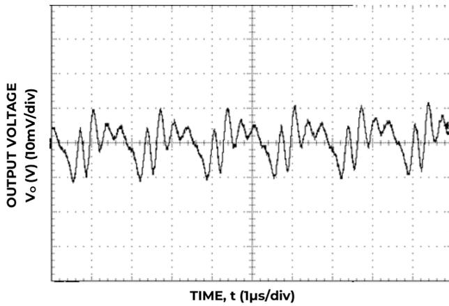
Figure 9. Typical output ripple and noise (C<sub>o</sub>=10μF ceramic, V<sub>IN</sub> = 12V, I<sub>o</sub> = I<sub>o,max</sub>).
