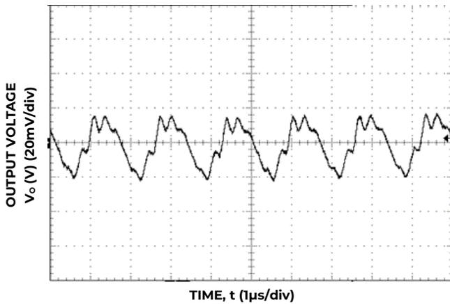
Figure 27. Typical output ripple and noise
