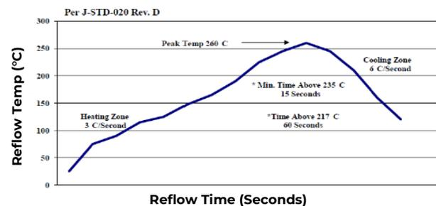
Figure 51. Recommended linear reflow profile using Sn/Ag/Cu solder.
