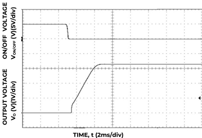
Figure 29. Typical Start-up Using On/Off Voltage (I<sub>o</sub> = I<sub>o,max</sub>).
