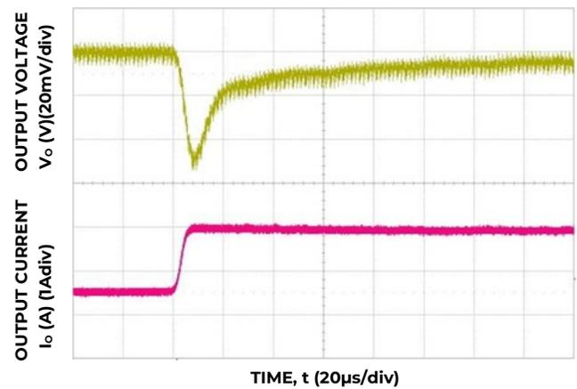
Figure 22. Transient Response to Dynamic Load Change from 50% to 100% at 12V<sub>in</sub>, C<sub>out</sub>=2x47µF, C<sub>Tune</sub>=2700pF, R<sub>Tune</sub>=267
