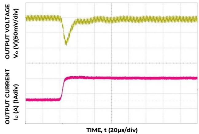
Figure 34. Transient Response to Dynamic Load Change from 50% to 100% at 12V<sub>in</sub>, C<sub>out</sub>=1x47µF, C<sub>Tune</sub>=820pF & R<sub>Tune</sub>=267
