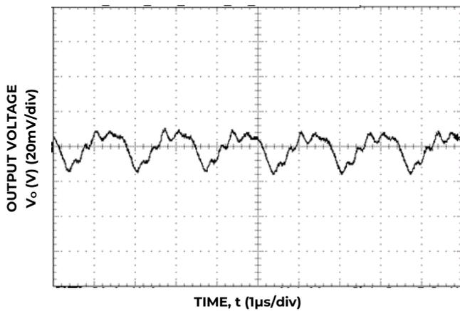
Figure 21. Typical output ripple and noise (C<sub>o</sub>=10µF ceramic, V<sub>IN</sub> = 12V, I<sub>o</sub> = I<sub>o,max</sub>).
