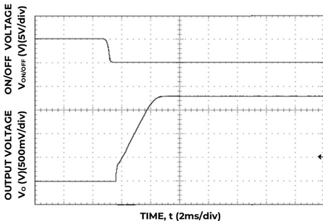
Figure 17. Typical Start-up Using On/Off Voltage (I<sub>o</sub> = I<sub>o,max</sub>).
