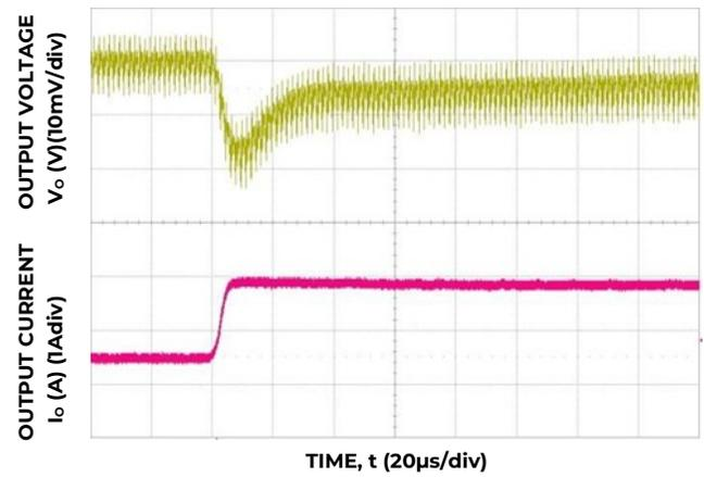
Figure 16. Transient Response to Dynamic Load Change from 50% to 100% at 12V<sub>in</sub>, C<sub>out</sub>=1x47μF+1x330μF, C<sub>Tune</sub>=10nF & R<sub>Tune</sub>=267
