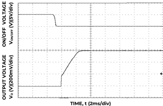
Figure 5. Typical Start-up Using On/Off Voltage (I<sub>o</sub> = I<sub>o,max</sub>).
