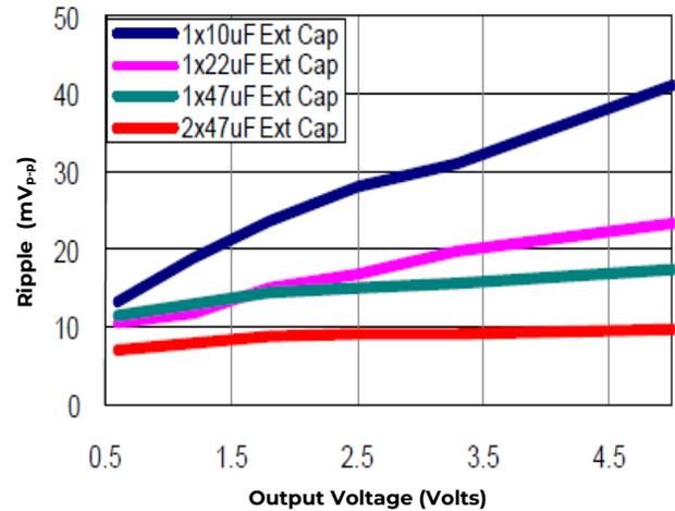
**Figure 38. Output ripple voltage for various output voltages with external 1x10  $\mu\text{F}$ , 1x22  $\mu\text{F}$ , 1x47  $\mu\text{F}$  or 2x47  $\mu\text{F}$  ceramic capacitors at the output (3A load). Input voltage is 12V.**
