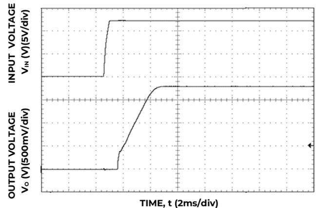
Figure 18. Typical Start-up Using Input Voltage (V<sub>IN</sub> = 12V, I<sub>o</sub> = I<sub>o,max</sub>).
