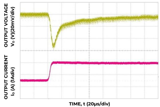
Figure 28. Transient Response to Dynamic Load Change from 50% to 100% at 12V<sub>in</sub>, C<sub>out</sub>=2x47µF, C<sub>Tune</sub>=2200pF, R<sub>Tune</sub>=267
