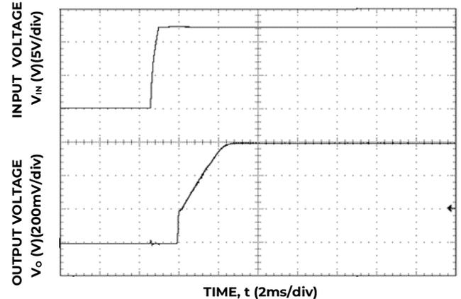
Figure 6. Typical Start-up Using Input Voltage (V<sub>IN</sub> = 12V, I<sub>o</sub> = I<sub>o,max</sub>).
