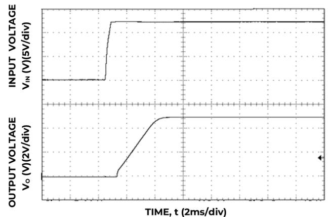
Figure 36. Typical Start-up Using Input Voltage
