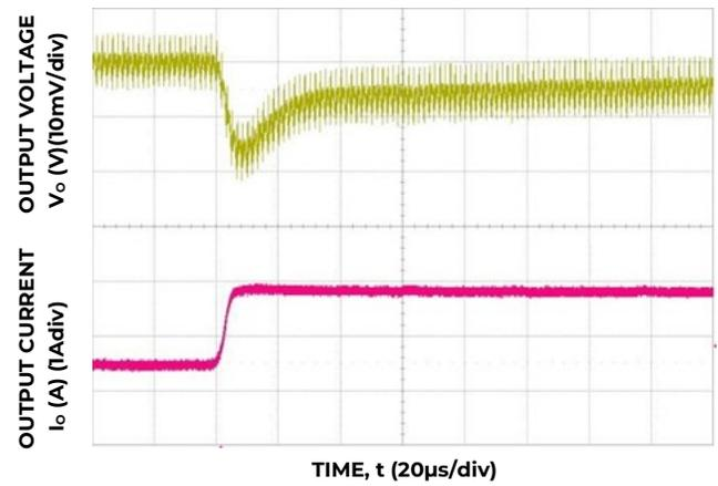
Figure 10. Transient Response to Dynamic Load Change from 50% to 100% at 12V<sub>in</sub>, C<sub>out</sub>=1x47μF+1x330μF, C<sub>Tune</sub>=10nF, R<sub>Tune</sub>=267
