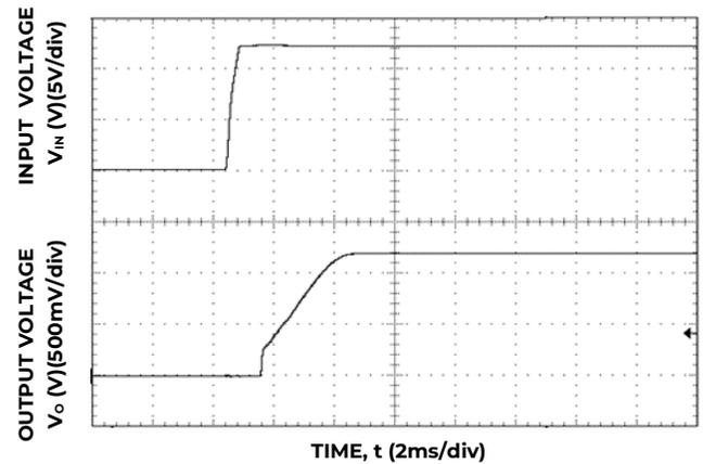
Figure 12 Typical Start-up Using Input Voltage (V<sub>IN</sub> = 12V, I<sub>o</sub> = I<sub>o,max</sub>).
