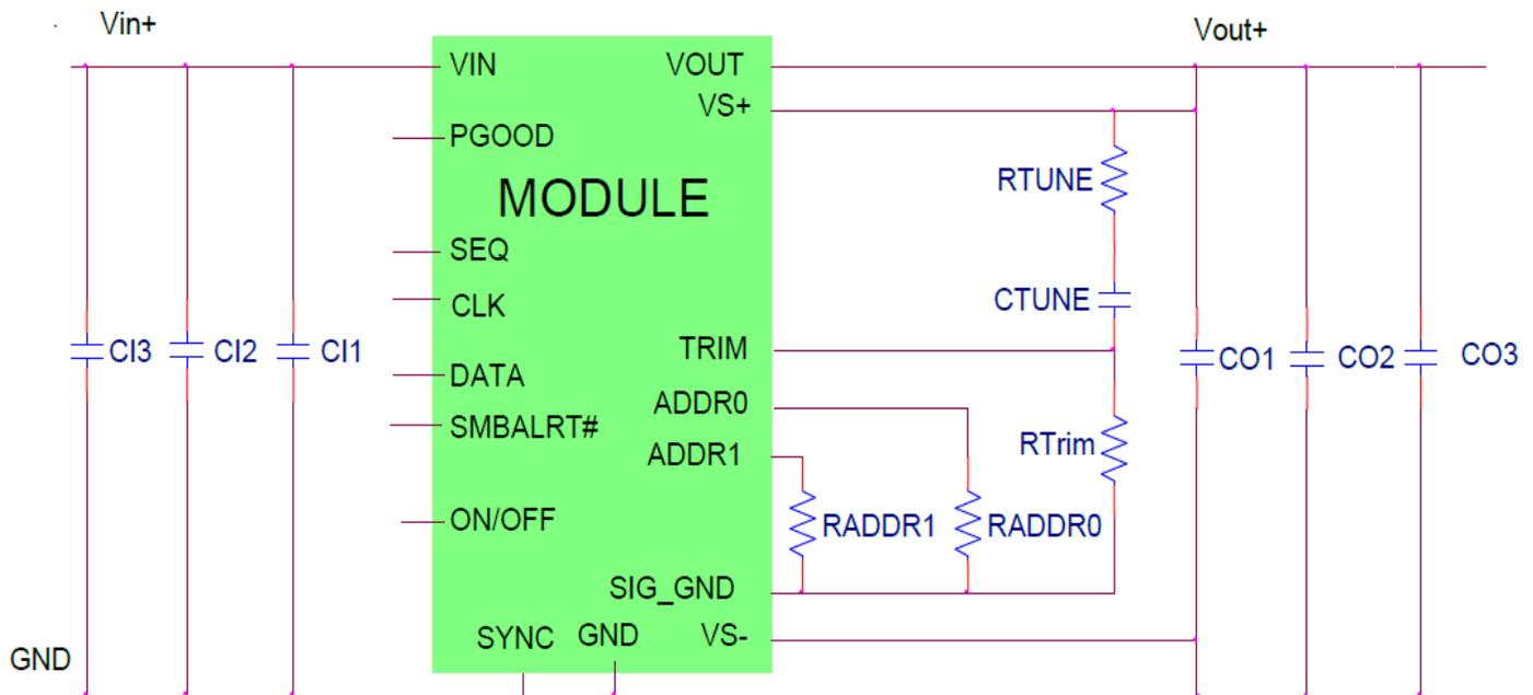
CI1 Decoupling cap - 1x0.047 $\mu$ F/16V ceramic capacitor (e.g. Murata LLL185R71C473MA01)
