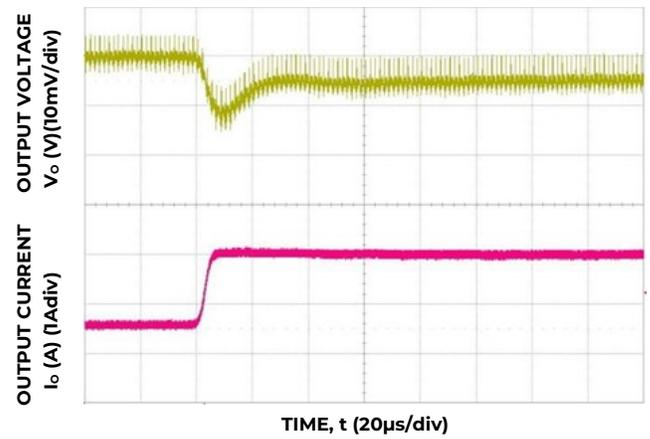
Figure 4. Transient Response to Dynamic Load Change from 50% to 100% at 12V<sub>in</sub>, C<sub>out</sub>=1x47µF+2x330µF, C<sub>Tune</sub>=27nF, R<sub>Tune</sub>=180
