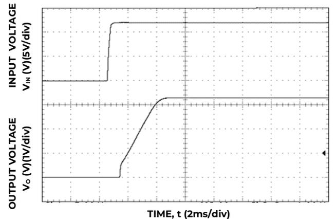
Figure 30. Typical Start-up Using Input Voltage
