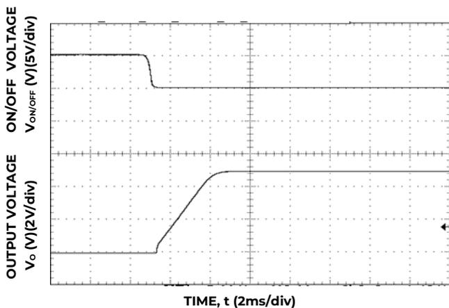
Figure 35. Typical Start-up Using On/Off Voltage (I<sub>o</sub> = I<sub>o,max</sub>).
