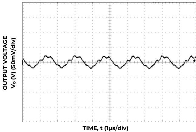
Figure 33. Typical output ripple and noise
