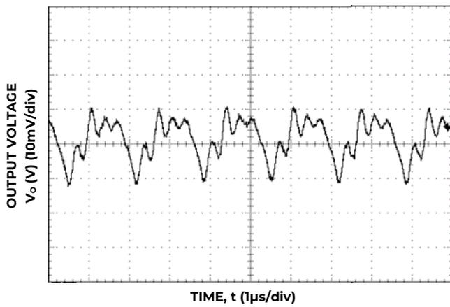
Figure 15. Typical output ripple and noise (C<sub>o</sub>=10μF ceramic, V<sub>IN</sub> = 12V, I<sub>o</sub> = I<sub>o,max</sub>).
