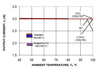
Figure 32. Derating Output Current verses Ambient Temperature and Airflow.
