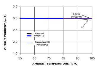
Figure 8. Derating Output Current verses Ambient Temperature and Airflow.
