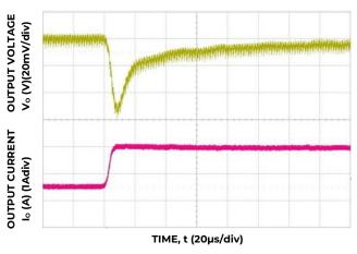
Figure 28. Transient Response to Dynamic Load Change from 50% to 100% at 12V<sub>in</sub>, C<sub>out</sub>=2x47µF, C<sub>Tune</sub>=2200pF, R<sub>Tune</sub>=267
