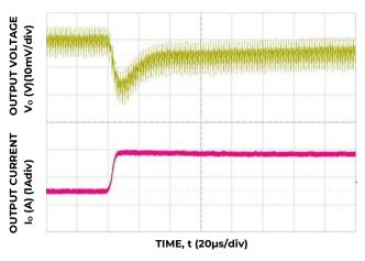
Figure 16. Transient Response to Dynamic Load Change from 50% to 100% at  $12V_{in}$ ,  $C_{out}=1x47\mu F+1x330\mu F$ ,  $C_{Tune}=10nF$  &  $R_{Tune}=267$
