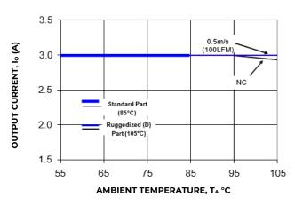
Figure 14. Derating Output Current verses Ambient Temperature and Airflow.
