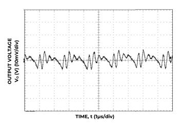
Figure 3. Typical output ripple and noise  $(C_0=10\mu F \text{ ceramic}, V_{IN}=12V, I_0=I_{0,max}).$
