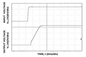
Figure 30. Typical Start-up Using Input Voltage  $(V_{\text{IN}}=12V,\,I_{\text{o}}=I_{\text{o,max}}).$
