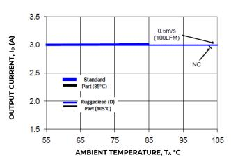
Figure 20. Derating Output Current verses Ambient Temperature and Airflow.
