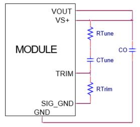
Figure. 47. Circuit diagram showing connection of  $R_{\text{TUNE}}$  and  $C_{\text{TUNE}}$  to tune the control loop of the module.
