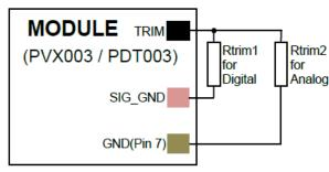
Figure 46. Connections to support either Analog or Digital PicoDLynx on the same layout.
