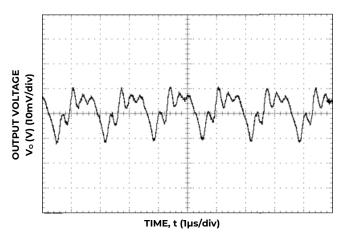
Figure 15. Typical output ripple and noise  $(C_0=10\mu F \text{ ceramic}, V_{IN}=12V, I_0=I_{0,max})$ .
