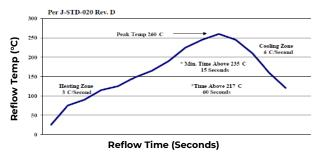
Figure 51. Recommended linear reflow profile using Sn/Ag/Cu solder.
