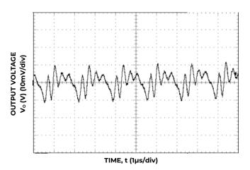
Figure 9. Typical output ripple and noise  $(C_0=10\mu F \text{ ceramic}, V_{IN}=12V, I_0=I_{0,max}).$
