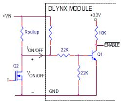
Figure 39. Circuit configuration for using positive On/Off logic.
