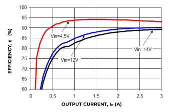
Figure 19. Converter Efficiency verses output current
