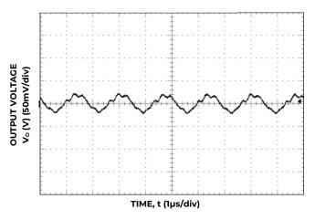
Figure 33. Typical output ripple and noise  $(C_0=10\mu F \text{ ceramic}, V_{IN}=12V, I_0=I_{0,max_i}).$
