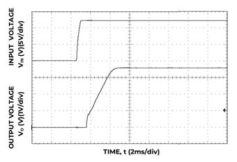
Figure 24. Typical Start-up Using Input Voltage  $(V_{\text{IN}}=12V,\,I_{\text{o}}=I_{\text{o,max}}).$
