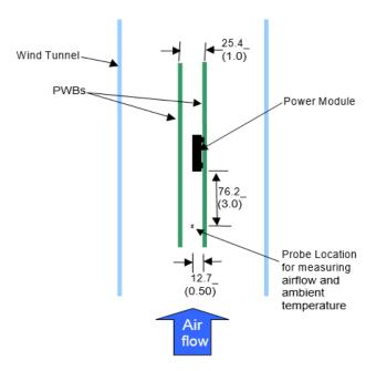
Figure 49. Thermal Test Setup.
