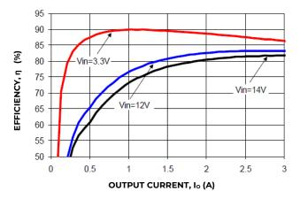
Figure 7. Converter Efficiency verses output current
