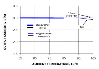
Figure 2. Derating Output Current verses Ambient Temperature and Airflow.
