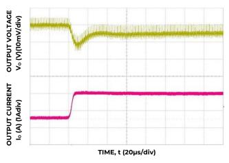
Figure 4. Transient Response to Dynamic Load Change from 50% to 100% at  $12V_{in}$ ,  $C_{out}=1x47\mu F+2x330\mu F$ ,  $C_{Tune}=27nF$ ,  $R_{Tune}=180$
