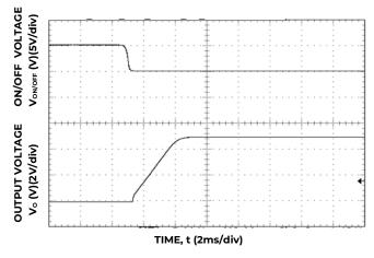
Figure 35. Typical Start-up Using On/Off Voltage ( $I_0 = I_{o,max}$ ).
