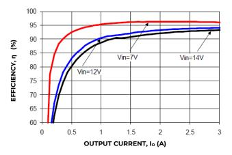
Figure 31. Converter Efficiency verses output current
