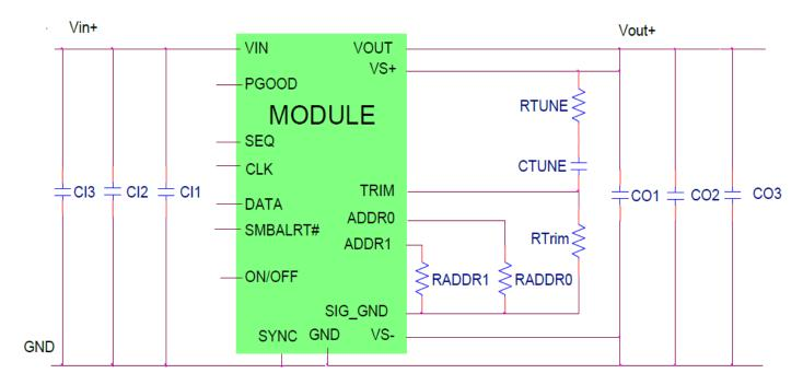
CII Decoupling cap - 1x0.047µF/16V ceramic capacitor (e.g. Murata LLL185R71C473MA01)
