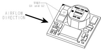
Figure 50. Preferred airflow direction and location of hot- spot of the module (T<sub>ref</sub>).
