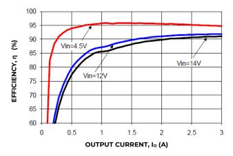
Figure 25. Converter Efficiency verses output current
