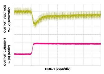
Figure 10. Transient Response to Dynamic Load Change from 50% to 100% at 12 $V_{in}$ ,  $C_{out}$ =1x47 $\mu$ F+1x330 $\mu$ F,  $C_{Tune}$ =10nF,  $R_{Tune}$ =267
