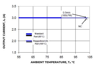
Figure 26. Derating Output Current verses Ambient Temperature and Airflow.
