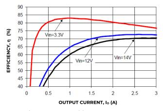
Figure 1. Converter Efficiency verses output current
