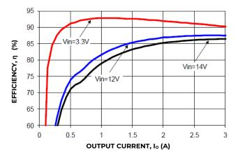
Figure 13. Converter Efficiency verses output current
