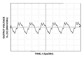
Figure 27. Typical output ripple and noise  $(C_0=10\mu F \text{ ceramic}, V_{IN}=12V, I_0=I_{0,max_i}).$
