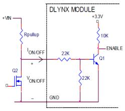
Figure 40. Circuit configuration for using negative On/Off logic.
