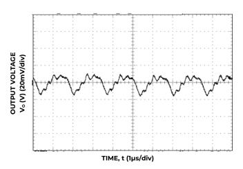
Figure 21. Typical output ripple and noise  $(C_0=10\mu F \text{ ceramic}, V_{IN}=12V, I_0=I_{0,max}).$
