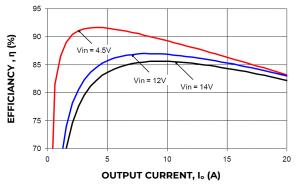
Figure 7. Converter Efficiency versus Output Current.
