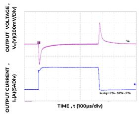
Figure 22. Transient Response to Dynamic Load Change from 0% to 50% to 0% with  $V_{\rm IN}$ =12V.
