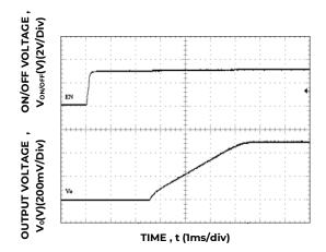
Figure 35. Typical Start-up Using On/Off Voltage ( $I_0 = I_{o,max}$ ).
