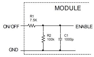
Figure 47. Remote On/Off Implementation. Resistor R1 is absent in the -49Z option modules.
