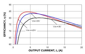
Figure 1. Converter Efficiency versus Output Current.
