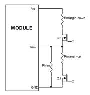
Figure 50. Circuit Configuration for margining Output voltage.
