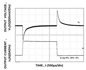
Figure 40. Transient Response to Dynamic Load Change from 0% to 50% to 0% with  $V_{\rm IN}$ =12V.
