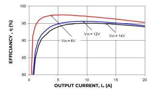
Figure 31. Converter Efficiency versus Output Current.
