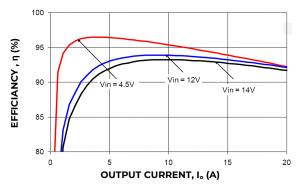
Figure 25. Converter Efficiency versus Output Current.
