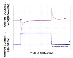
Figure 28. Transient Response to Dynamic Load Change from 0% to 50% to 0% with  $V_{\text{IN}}$ =12V.
