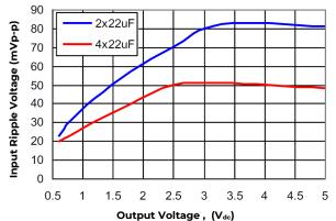
Figure 46. Input ripple voltage for various output voltages with 2x22  $\mu F$  or 4x22  $\mu F$  ceramic capacitors at the input (20A load). Input voltage is 12V.
