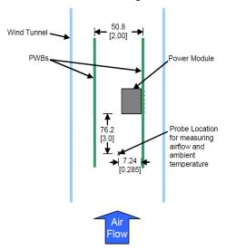
Figure 52. Thermal Test Set-up.
