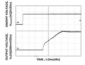
Figure 5. Typical Start-up Using On/Off Voltage  $(I_0 = I_{0,max})$ .
