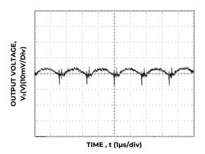
Figure 3. Typical output ripple and noise  $(V_{\text{IN}} = 9V, \ I_o = I_{o,\text{max}}).$
