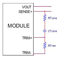
Figure. 51. Circuit diagram showing connection of  $R_{\text{TUME}}$  and  $C_{\text{TUNE}}$  to tune the control loop of the module.
