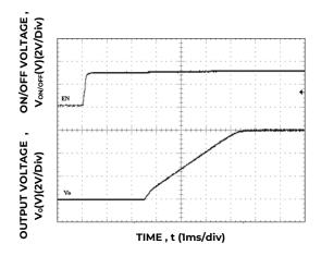
Figure 41. Typical Start-up Using On/Off Voltage ( $I_o = I_{o,max}$ ).
