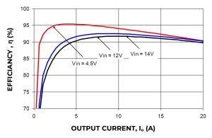
Figure 19. Converter Efficiency versus Output Current.
