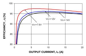
Figure 37. Converter Efficiency versus Output Current.
