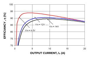
Figure 13. Converter Efficiency versus Output Current.
