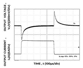
Figure 34. Transient Response to Dynamic Load Change from 0% to 50% to 0% with  $V_{\rm IN}$ =12V.
