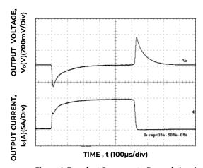
Figure 4. Transient Response to Dynamic Load Change from 0% to 50% to 0% with  $V_{\text{IN}}$ =9V.
