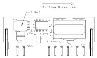
Figure 53. Temperature measurement location.
