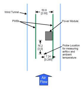
Figure 53. Thermal Test Set-up.
