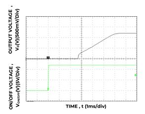
Figure 11. Typical Start-up Using On/Off Voltage ( $I_0 = I_{o,max}$ ).
