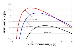
Figure 1. Converter Efficiency versus Output Current.
