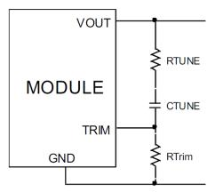
Figure. 52. Circuit diagram showing connection of  $R_{\text{TUNE}}$  and  $C_{\text{TUNE}}$  to tune the control loop of the module.
