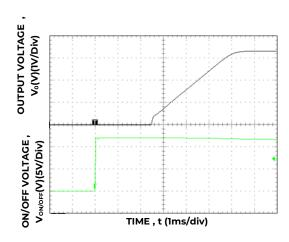
Figure 29. Typical Start-up Using On/Off Voltage  $(I_0 = I_{o,max})$ .
