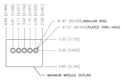
TO INCREASE COPPER ADHESION, ELLIPTICAL PADS CAN BE UTILIZED
