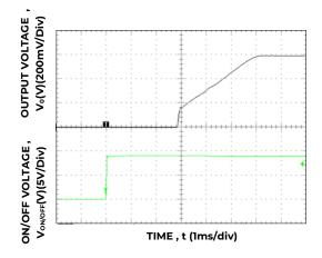
Figure 5. Typical Start-up Using On/Off Voltage  $(I_0 = I_{0,max})$ .
