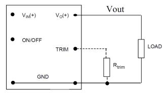
Figure 50. Circuit configuration for programming output voltage using an external resistor.
