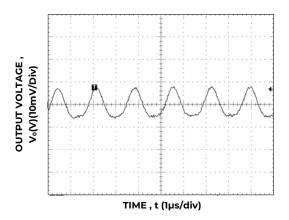
Figure 15. Typical output ripple and noise ( $V_{\rm IN}$  = 12V,  $I_{\rm o}$  = I  $_{\rm o,max}$ ).
