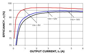
Figure 31. Converter Efficiency versus Output Current.
