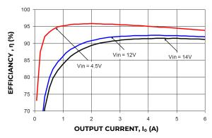
Figure 25. Converter Efficiency versus Output Current.
