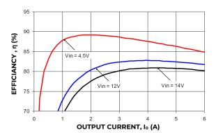
Figure 7. Converter Efficiency versus Output Current.
