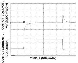
Figure 34. Transient Response to Dynamic Load Change from0% to 50% to 0% with V<sub>IN</sub>=12V.
