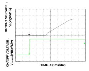
Figure 23. Typical Start-up Using On/Off Voltage ( $I_0 = I_{o,max}$ ).
