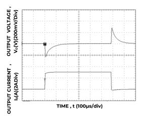
Figure 16. Transient Response to Dynamic Load Change from 0% to 50% to 0% with V<sub>IN</sub>=12V.
