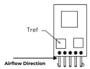
Figure 54. T<sub>ref</sub> Temperature measurement location.
