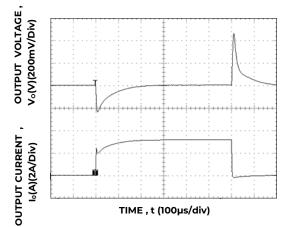
Figure 4. Transient Response to Dynamic Load Change from 0% to 50% to 0% with  $V_{\text{IN}}$ =9V.
