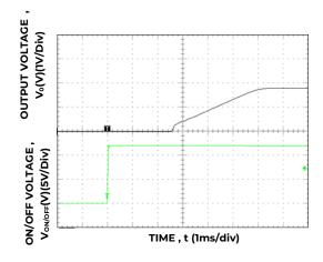
Figure 17. Typical Start-up Using On/Off Voltage ( $I_0 = I_{o,max}$ ).
