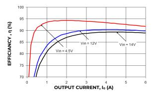
Figure 19. Converter Efficiency versus Output Current.
