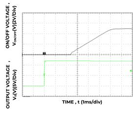
Figure 41. Typical Start-up Using On/Off Voltage  $(I_0 = I_{o,max})$ .
