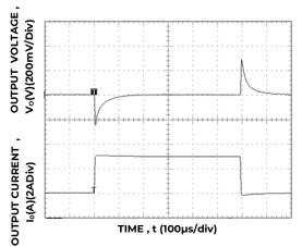
Figure 40. Transient Response to Dynamic Load Change from0% to 50% to 0% with V<sub>IN</sub>=12V.
