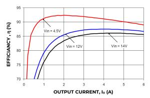
Figure 13. Converter Efficiency versus Output Current.
