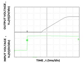
Figure 42. Typical Start-up Using Input Voltage ( $V_{\text{IN}}$  = 12V,  $I_{\text{o}}$  =  $I_{\text{o,max}}$ ).
