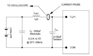
Figure 43. Input Reflected Ripple Current Test Setup.
