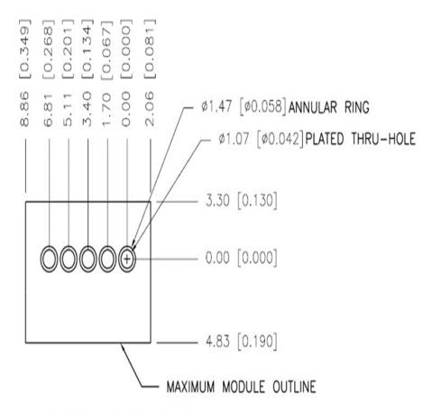
TO INCREASE COPPER ADHESION, ELLIPTICAL PADS CAN BE UTILIZED
