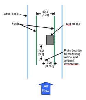
Figure 53. Thermal Test Setup.
