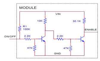
Figure 48. Remote On/Off Implementation. Resistor R1 is absent in the -49Z option module.
