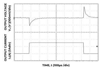
Figure 34. Transient Response to Dynamic Load Change from 0% to 50% to 0% with  $V_{\text{IN}}$ =12V.
