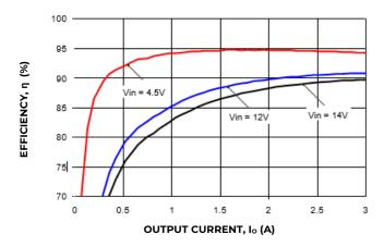
Figure 19. Converter Efficiency versus Output Current.
