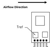
Figure 54. T<sub>ref</sub> Temperature measurement location.
