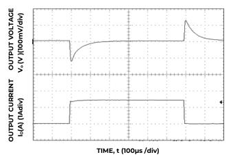
Figure 16. Transient Response to Dynamic Load Change from 0% to 50% to 0% with  $V_{\text{IN}}$ =12V.
