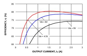
Figure 1. Converter Efficiency versus Output Current
