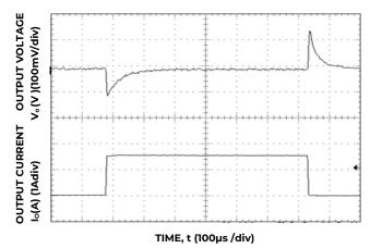
Figure 40. Transient Response to Dynamic Load Change from 0% to 50% to 0% with V<sub>IN</sub>=12V.
