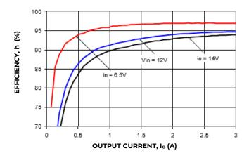
Figure 31. Converter Efficiency versus Output Current.
