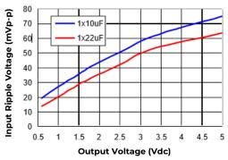
Figure 46. Input ripple voltage for various output voltages with 1x10 µF or 1x22 µF ceramic capacitors at the input (3A load). Input voltage is 12V
