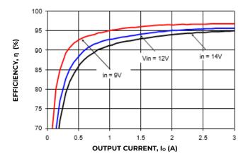
Figure 37. Converter Efficiency versus Output Current.
