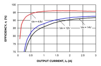
Figure 25. Converter Efficiency versus Output Current.
