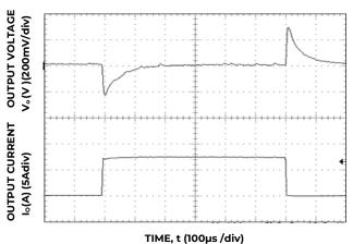
Figure 22. Transient Response to Dynamic Load Change from 0% to 50% to 0% with V<sub>IN</sub>=12V.
