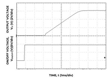
Figure 41. Typical Start-up Using On/Off Voltage (I<sub>o</sub> = I<sub>o,max</sub>).
