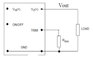
Figure 50. Circuit configuration for programming output voltage using an external resistor.
