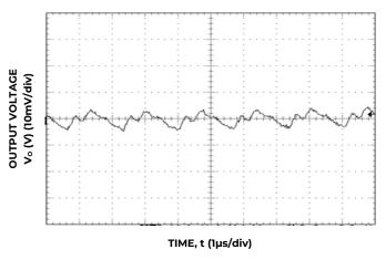
Figure 9. Typical output ripple and noise (V  $_{\mbox{\scriptsize IN}}$  = 12V,  $I_{\mbox{\scriptsize o}}$  = I  $_{\mbox{\scriptsize o,max}}$ ).
