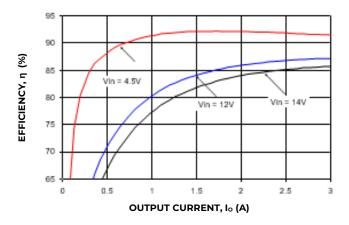
Figure 13. Converter Efficiency versus Output Current.
