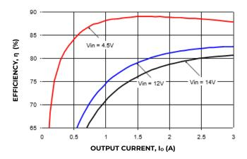
Figure 7. Converter Efficiency versus Output Current
