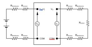
Figure 45. Output Voltage and Efficiency Test Setup.
