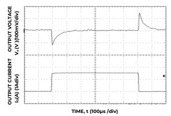
Figure 28. Transient Response to Dynamic Load Change from 0% to 50% to 0% with  $V_{\rm IN}$ =12V.
