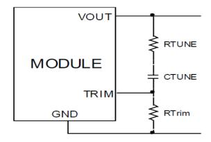
Figure. 52. Circuit diagram showing connection of  $R_{\text{TUNE}}$  and  $C_{\text{TUNE}}$  to tune the control loop of the module.
