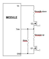
Figure 51. Circuit Configuration for margining Output voltage.
