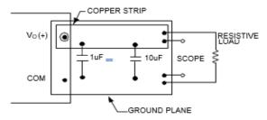
Figure 44. Output Ripple and Noise Test Setup
