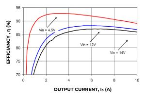
Figure 13. Converter Efficiency versus Output Current.
