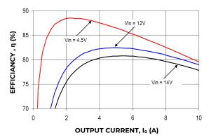
Figure 7. Converter Efficiency versus Output Current.
