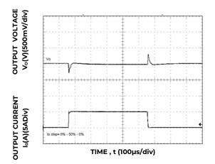
Figure 22. Transient Response to Dynamic Load Change from 0% to 50% to 0% with  $V_{\text{IN}}$ =12V.
