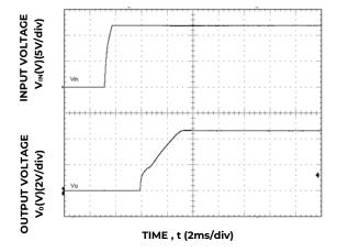
Figure 36. Typical Start-up Using Input Voltage  $(V_{\text{IN}} = 12V, \ J_{\text{o}} = I_{\text{o,max}}).$
