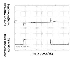
Figure 34. Transient Response to Dynamic Load Change from 0% to 50% to 0% with  $V_{\text{IN}}$ =12V.
