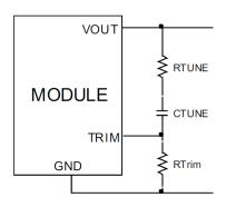
Figure. 52. Circuit diagram showing connection of  $R_{\text{TUME}}$  and  $C_{\text{TUNE}}$  to tune the control loop of the module.
