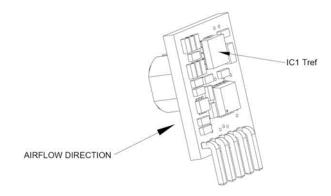
Figure 54. Tref Temperature measurement location.
