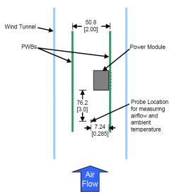
Figure 53 Thermal Test Set-up.
