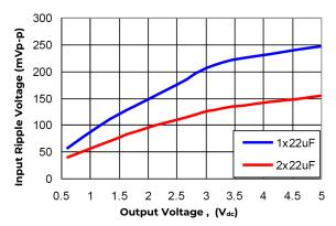
Figure 4. Input ripple voltage for various output voltages with 1x22 µF or 2x22 µF ceramic capacitors at the input (10A load).
