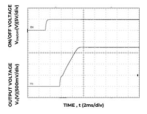
Figure 17. Typical Start-up Using On/Off Voltage  $(I_0 = I_{0,max})$ .
