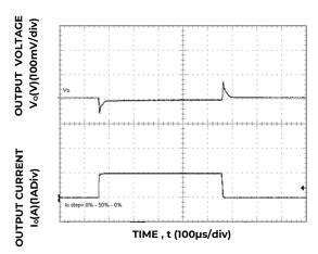
Figure 40. Transient Response to Dynamic Load Change from 0% to 50% to 0% with  $V_{\text{IN}}$ =12V.
