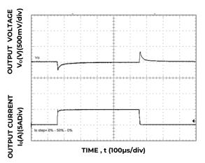
Figure 16. Transient Response to Dynamic Load Change from 0% to 50% to 0% with V<sub>IN</sub>=12V.
