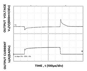
Figure 4. Transient Response to Dynamic Load Change from 0% to 50% to 0% with V<sub>IN</sub>=9V.
