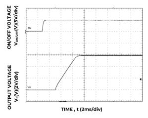
Figure 41. Typical Start-up Using On/Off Voltage ( $I_0 = I_{o,max}$ ,  $V_{in} = 12V$ ).
