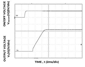
Figure 29. Typical Start-up Using On/Off Voltage (I $_{\rm o,max}$  ).
