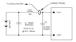
Figure 43. Input Reflected Ripple Current Test Setup.
