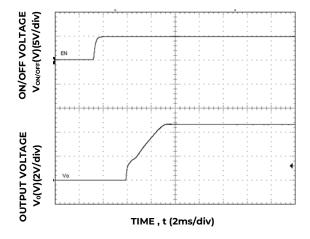
Figure 35. Typical Start-up Using On/Off Voltage ( $I_0 = I_{0,max}$ ).
