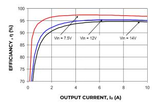
Figure 31. Converter Efficiency versus Output Current.
