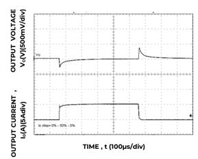
Figure 10. Transient Response to Dynamic Load Change from 0% to 50% to 0% with  $V_{\text{IN}}$ =12V.
