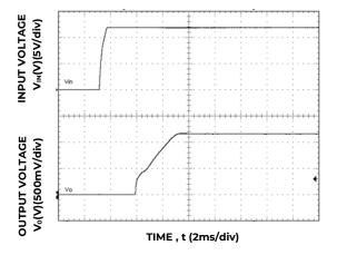
Figure 12. Typical Start-up Using Input Voltage  $(V_{IN} = 9V, I_o = I_{o,max}).$
