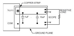
Figure 44. Output Ripple and Noise Test Setup.
