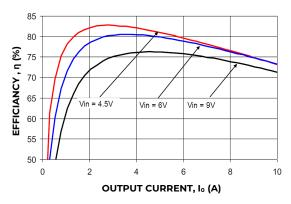
Figure 1. Converter Efficiency versus Output Current.
