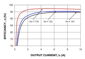
Figure 37. Converter Efficiency versus Output Current.
