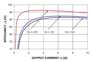
Figure 25. Converter Efficiency versus Output
