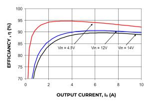
Figure 19. Converter Efficiency versus Output Current.
