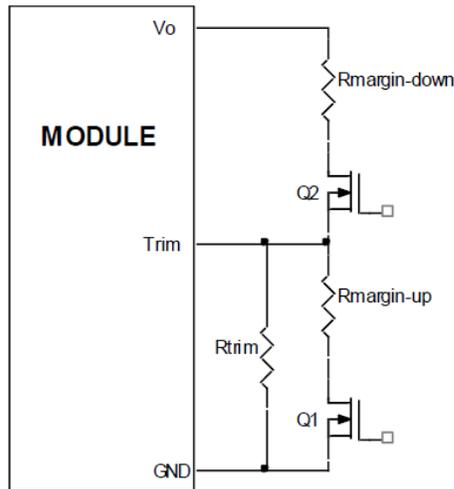
Figure 9. Circuit Configuration for margining Output voltage.
