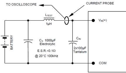
**Figure 1. Input Reflected Ripple Current Test Setup.**
