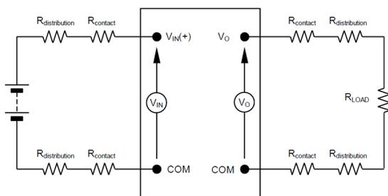
**Figure 3. Output Voltage and Efficiency Test Setup.**
