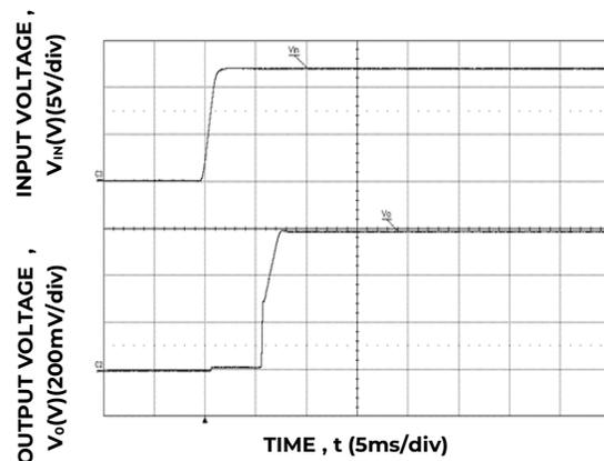
Figure 6. Typical Start-up Using Input Voltage ( $V_{IN} = 12V, C_{ext} = 22\mu F, I_o = I_{o,max}$ ).
