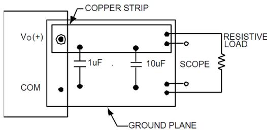
**Figure 2. Output Ripple and Noise Test Setup.**
