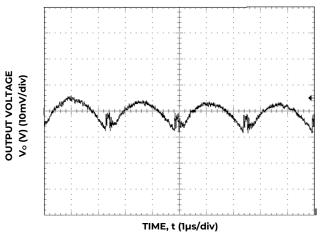
Figure 3. Typical output ripple and noise (C<sub>0</sub>=6x47  $\mu$ F ceramic, V<sub>IN</sub> = 12V, I<sub>0</sub> = I<sub>0,max</sub>).
