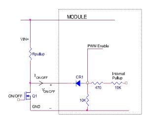
Figure 21. Circuit configuration for using positive On/Off logic.
