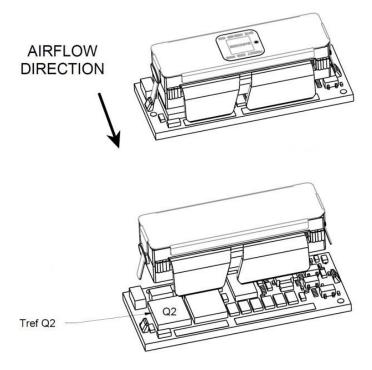
Figure 30. Preferred airflow direction and location of hotspot of the module ( $T_{\rm ref}$ ).
