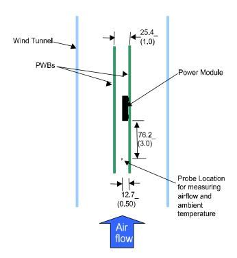
Figure 29. Thermal Test Setup.
