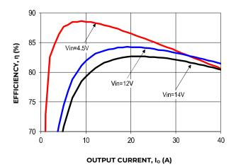
Figure 1. Converter Efficiency versus Output Current.
