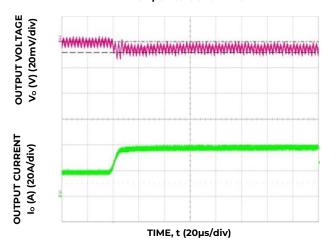
Figure 4. Transient Response to Dynamic Load Change from 50% to 100% at 12V  $_{in}$  ,  $C_{out}$  = 12x680  $\mu F$  +6x47  $\mu F$  , C<sub>Tune</sub>=47nF, R<sub>Tune</sub>=180 ohms
