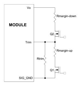
Figure 25. Circuit Configuration for margining Output voltage.
