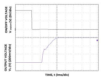
Figure 5. Typical Start-up Using On/Off Voltage
