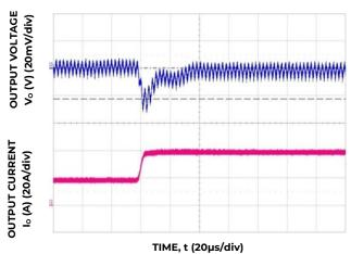
Figure 10. Transient Response to Dynamic Load Change from 50% to 100% at 12Vin, Cout= 6x330µF, Ctune=12nF, Rtune=200 ohms
