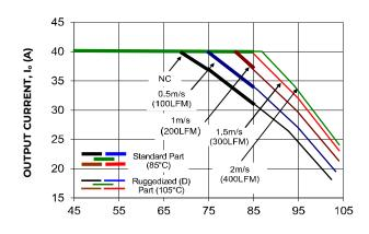
AMBIENT TEMPERATURE, TA °C Figure 2. Derating Output Current versus Ambient Temperature and Airflow.
