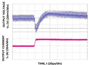
Figure 16. Transient Response to Dynamic Load Change from 50% to 100% at  $12V_{in}$ ,  $C_{out}$ =  $6x330\mu F$ ,  $C_{Tune}$ =5.6nF &  $R_{Tune}$ =220 ohms.
