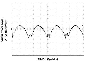
Figure 9. Typical output ripple and noise ( $C_0=6x47\mu F$  ceramic,  $V_{IN}=12V$ ,  $I_0=I_{o,max}$ ).
