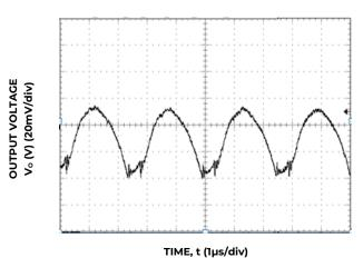
Figure 15. Typical output ripple and noise ( $C_0=6x47\mu F$  ceramic,  $V_{IN}=12V$ ,  $I_0=I_{0,max}$ ).
