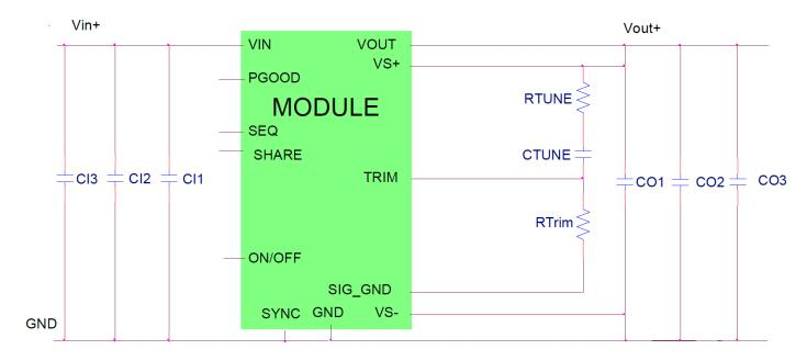
CII Decoupling cap - 1x0.01µF/16V ceramic capacitor (e.g. Murata LLL185R71E103MA01)
