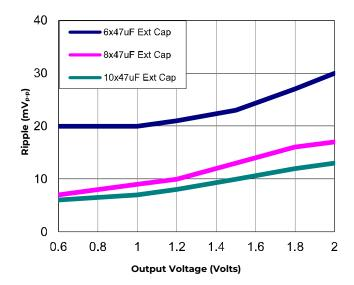
Figure 20. Output ripple voltage for various output voltages with external 6x47  $\mu$ F, 8x47  $\mu$ F or 10x47  $\mu$ F ceramic capacitors at the output (40A load). Input voltage is 12V. Scope Bandwidth limited to 20MHz
