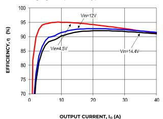
Figure 13 Converter Efficiency versus Output Current.
