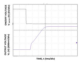
Figure 17. Typical Start-up Using On/Off Voltage  $(I_0 = I_{o,max})$ .
