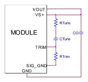
Figure. 28. Circuit diagram showing connection of  $R_{\text{TUNE}}$  and  $C_{\text{TUNE}}$  to tune the control loop of the module.
