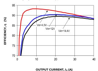
Figure 7. Converter Efficiency versus Output Current.
