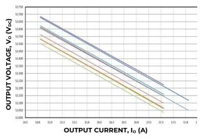
Figure 2. Output current limit profile (0° - 50°C)
