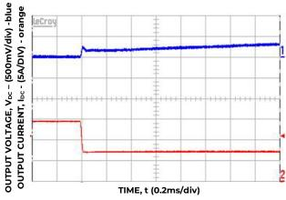
Figure 10. 54V Transient response 50% load step (100 - 50%)
