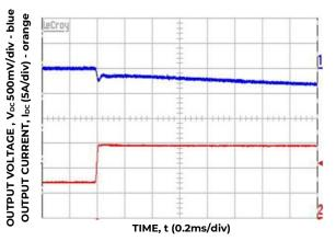
Figure 9. 54V Transient response 50% load step (50 – 100%)
