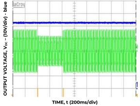
Figure 11. 30% dip ride-through  $V_{\text{IN}}$  240  $V_{\text{AC}}$
