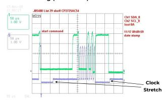
Figure 1. Example waveforms showing clock stretching.
