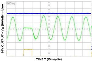
Figure 8.  $\frac{1}{2}$  cycle ride-through  $V_{IN}$  240  $V_{AC}$
