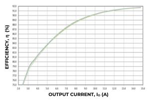
Figure 1. Efficiency V<sub>IN</sub>: 240V, Freq: 60Hz
