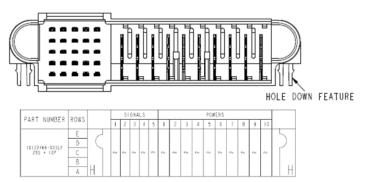
With respect to signals "3" in Columns 5, refers to the shortest level signal pin; the "shortest" pins are the "last to make, first to break" in the mating sequence
