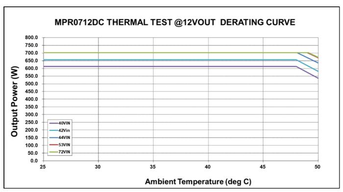
The curves for  $40V_{\text{IN}}$  and  $42V_{\text{IN}}$  are only for DCX.
