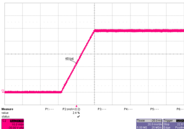
Figure 9. 48V DC soft start, full load, V IN =230V AC
