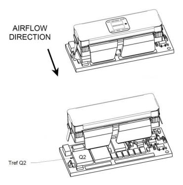
Figure 31. Preferred airflow direction and location of hotspot of the module (T<sub>ref</sub>).
