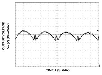
Figure 3. Typical output ripple and noise ( $C_0$ =6x47 $\mu$ F ceramic,  $V_{IN}$  = 12V,  $I_o$  =  $I_{o,max}$ ).
