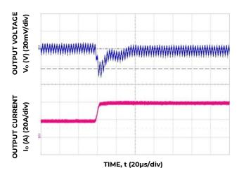
Figure 10. Transient Response to Dynamic Load Change from 50% to 100% at 12V<sub>in</sub>, C<sub>out</sub>= 6x330uF, C<sub>Tune</sub>=12nF, R<sub>Tune</sub>=200 ohms
