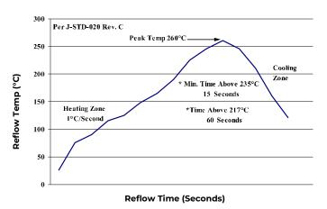
Figure 32. Recommended linear reflow profile using Sn/Ag/Cu solder.
