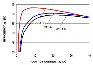
Figure 7. Converter Efficiency versus Output Current.
