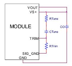
Figure. 28. Circuit diagram showing connection of  $R_{\text{TUNE}}$  and  $C_{\text{TUNE}}$  to tune the control loop of the module.
