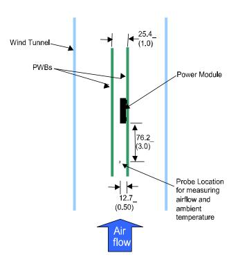
Figure 30. Thermal Test Setup.
