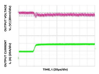
Figure 4. Transient Response to Dynamic Load Change from 50% to 100% at 12V<sub>in</sub>, C<sub>out</sub>= 12x680uF +6x47uF C<sub>Tune</sub>=47nF, R<sub>Tune</sub>=180 ohms
