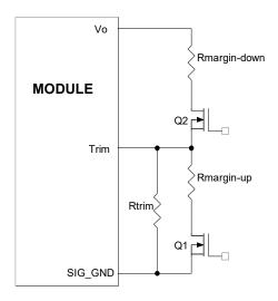
Figure 25. Circuit Configuration for margining Output voltage.
