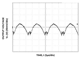
Figure 9. Typical output ripple and noise ( $C_0=6x47\mu F$  ceramic,  $V_{IN}=12V$ ,  $I_0=I_{o,max}$ ).
