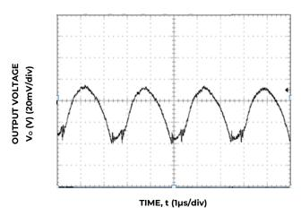
Figure 15. Typical output ripple and noise ( $C_0=6x47\mu F$  ceramic,  $V_{IN}=12V$ ,  $I_0=I_{0,max}$ ).
