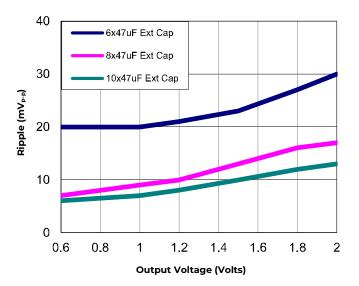
Figure 20. Output ripple voltage for various output voltages with external 6x47  $\mu$ F, 8x47  $\mu$ F or 10x47  $\mu$ F ceramic capacitors at the output (40A load). Input voltage is 12V. Scope Bandwidth limited to 20MHz
