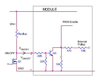
Figure 22. Circuit configuration for using negative On/Off logic.
