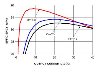
Figure 1. Converter Efficiency versus Output Current.
