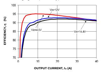
Figure 13 Converter Efficiency versus Output Current.
