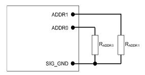
Figure 29. Circuit showing connection of resistors used to set the PMBus address of the module.
