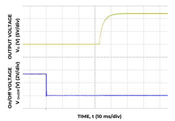
Figure 5.Typical Start-up Using Remote On/Off, negative logic version shown (  $V_{\rm IN}$  = 24V or 48V,  $I_{\rm o}$  =  $I_{\rm o,\ max}$ ).
