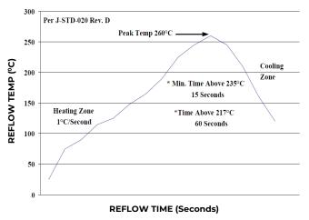
Figure 21. Recommended linear reflow profile using Sn/Ag/Cu solder
