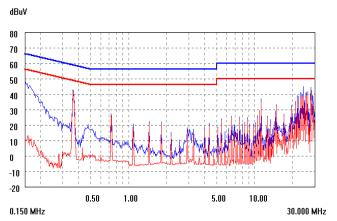
Figure 17. KHHD002A5B V<sub>in</sub>+ Line EMC signature using above filter, V<sub>in</sub>=48V, Blue=PK, Red=Avg.
