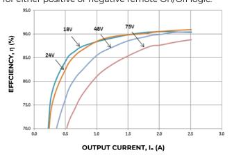
Figure 1. Converter Efficiency versus Output Current.
