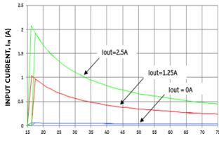
Figure 2. Converter Input Current versus Input Voltage.
