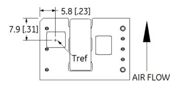
Figure 15. T<sub>ref</sub> Temperature Measurement Location.
