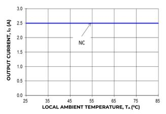
Figure 14. Output Current Derating for the Open Frame KHHD002A0B in the Transverse Orientation; Airflow Direction from V<sub>in</sub>(+) to V<sub>in</sub>(-); V<sub>in</sub> = 24V or 48V.
