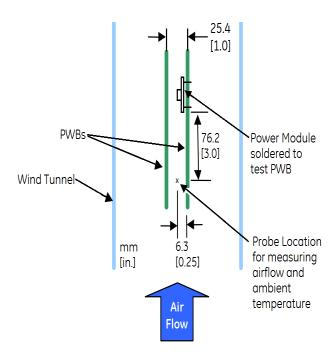
Figure 13. Thermal Test Setup.
