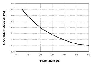
Figure 20. Time Limit, T<sub>lim</sub>, Curve Above 205°C Reflow.
