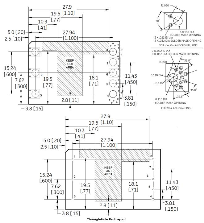
For .025  $\times$  .030 rectangular pin, use a .050 diameter plated through hole For .062 diameter pin, use a .076 diameter plated through hole.
