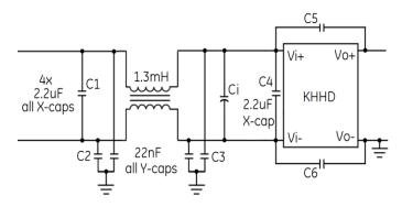
Figure 17. Suggested Configuration for EN55032 Class B.
