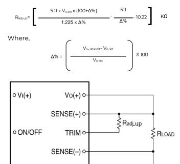
Figure 12. Circuit Configuration to Increase Output Voltage.
