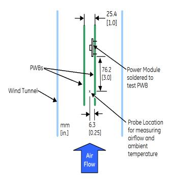
Figure 13. Thermal Test Setup.
