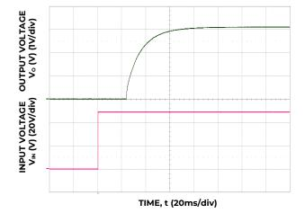
Figure 6. Typical Start-up Using Input Voltage ( $V_{IN} = 48V$ ,  $I_0 = I_{0, max}$ ).
