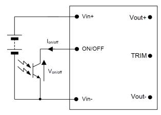
Figure 10. Circuit configuration for using Remote On/Off
