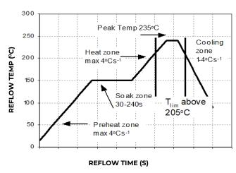
Figure 20. Recommended Reflow Profile for Sn/Pb solder.
