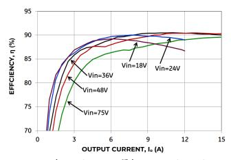
Figure 1. Converter Efficiency versus Output Current.
