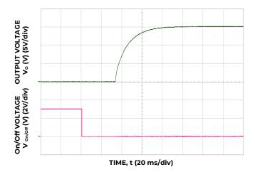
Figure 5.Typical Start-up Using Remote On/Off, negative logic version shown (V<sub>IN</sub> = 24V or 48V, I<sub>o</sub> = I<sub>o</sub>, max).
