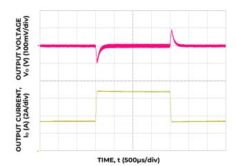
Figure 4. Transient Response to 0.1A/µS Dynamic load Change from 50% to 75% to 50% of full load, Vin=48V
