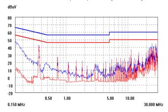
Figure 18. EMC signature using above filter, KHHD015A0.
