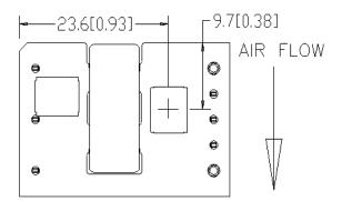
Figure 16. T<sub>ref</sub> Temperature Measurement Location.
