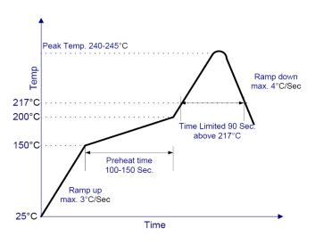
Figure 21. Recommended linear reflow profile using Sn/Ag/Cu solder.
