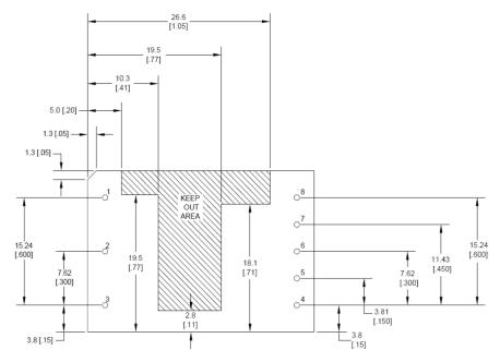
TH Recommended Pad Layout (Component Side View)
