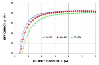
Figure 1. Converter Efficiency versus Output Current.
