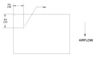
Figure 14. T<sub>ref</sub> Temperature Measurement Location for Module with Heatplate.
