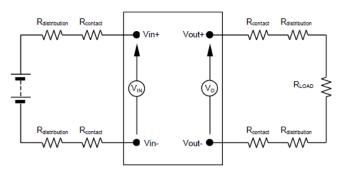
Figure 9. Output Voltage and Efficiency Test Setup.
