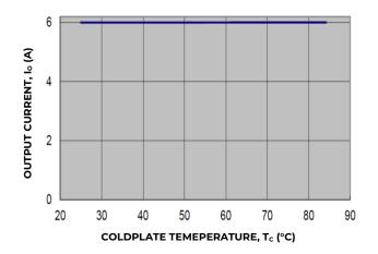
Figure 16b. Output Current Derating for the Module with Heatplate in a cold wall application; V<sub>in</sub> =48V.
