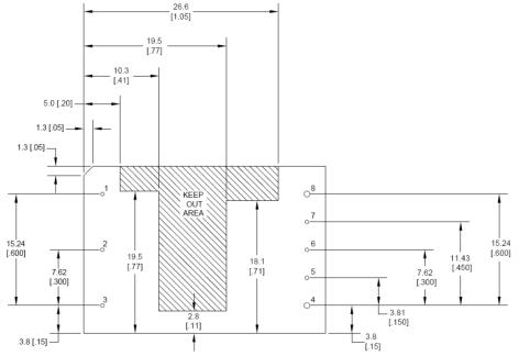
SMT Recommended Pad Layout (Component Side View)
