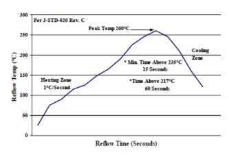
Figure 20. Recommended linear reflow profile using Sn/Ag/Cu solder.
