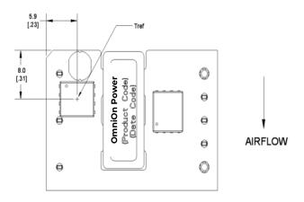
Figure 13. Tref Temperature Measurement Locations for Open Frame Module.
