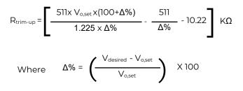
For example, to trim-up the output voltage of the module by 5% to 5.2V,  $R_{trim-up}$  is calculated is as follows:
