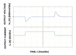
Figure 6. Dynamic Load Change Transient Response from 50 %to 75% to 50% of Full Load at Room Temperature and 48  $V_{IR}$ , 0.1A/uS,  $C_{o,ext}$  = 440 $\mu$ F.
