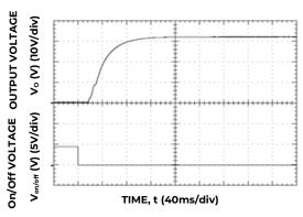
Figure 4. Typical Start-Up Using negative Remote On/Off;  $C_{o,ext} = 440 \mu F. \label{eq:control}$
