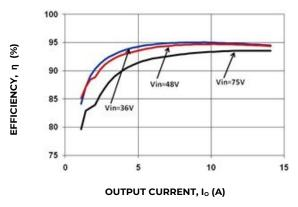
Figure 1. Converter Efficiency versus Output Current.
