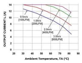
Figure 20. Derating Output Current vs. local Ambient temperature and Airflow, 0.5" Heat sink, V<sub>IN</sub> =48V, airflow from Vi(-) to Vi(+).
