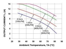
Figure 19. Derating Output Current vs. local Ambient temperature and Airflow, No Heat sink, V<sub>IN</sub> =48V, airflow from Vi(-) to Vi(+).
