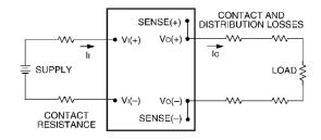
Figure 9. Output Voltage and Efficiency Test Setup.
