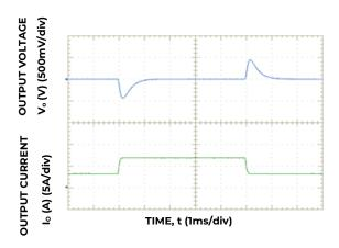
Figure 3. Dynamic Load Change Transient Response from 25% to 50% to 25% of Full Load at Room Temperature and 48 V<sub>IN</sub>;
