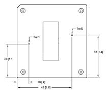
Figure 17. Case (TREF) Temperature Measurement Location (top view).
