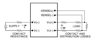
Figure 11. Effective Circuit Configuration for Single-Module Remote
