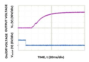
Figure 4. Typical Start-Up Using negative Remote On/Off; C<sub>0,ext</sub>= 440μF.
