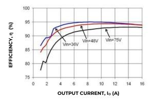
Figure 1. Converter Efficiency versus Output Current.
