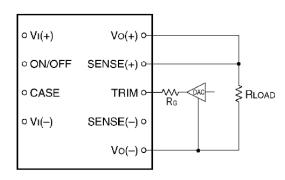
Figure 15. Circuit Configuration to Actively Adjust the Output Voltage
