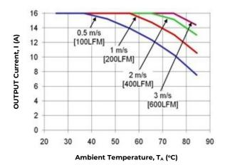
Figure 21. Derating Output Current vs. local Ambient temperature and Airflow, 1.0" Heatsink, V<sub>in</sub>=48V, airflow from Vi(-) to Vi(+).
