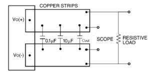
Figure 8. Output Ripple and Noise Test Setup
