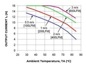
Figure 20. Derating Output Current vs. local Ambient temperature and Airflow, 0.5" Heat sink,  $V_{\rm in}$ =48V, airflow from Vi(-) to Vi(+).
