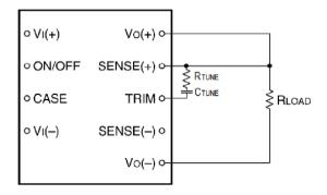
Figure 16. Circuit diagram showing connection of  $R_{\text{TUNE}}$  and  $C_{\text{TUNE}}$  to tune the control loop of the module.
