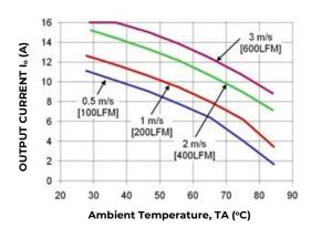
Figure 19. Derating Output Current vs. local Ambient temperature and Airflow, No Heat sink, Vin=48V, airflow from Vi(-) to Vi(+).
