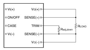
Figure 13. Circuit Configuration to Decrease Output Voltage.
