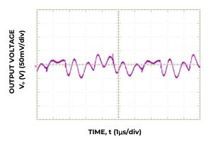
Figure 2. Typical output ripple and Noise at Room Temperature and  $48V_{in}$ ; lo =  $I_{o,max}$ ;  $C_{o,ext}$  =  $440\mu F$ .
