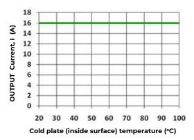
Figure 18. Output Power Derating for JRCW016A0R in Conduction cooling (cold plate) applications; Ta <70 $^{\circ}$ C adjacent to module;  $V_{\text{IN}} = V_{\text{IN,NOM}}$
