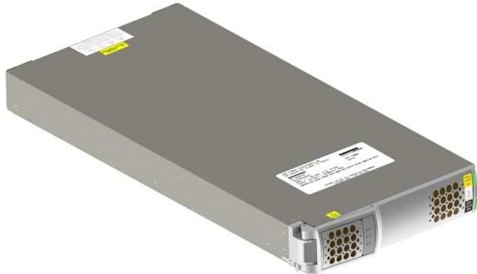
The OmniOn IR025H3R240ATEZ true three-phase rectifier efficiently transforms energy from any standard three-phase source into 240 volt DC power needed for industrial applications. The rectifier operates using three-phase input voltages from 320 to 530 VAC without the need of a neutral conductor. This means that one single rectifier can be used globally to meet all your 240V powering needs.
