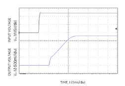
Figure 2. Typical Start-up using Input Voltage (Vin=12V, Vout = Vout, max, lout = lout, max)
