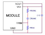
Figure 3. Circuit diagram showing connection of  $R_{\text{TUNE}}$  and  $C_{\text{TUNE}}$  to tune the control loop of the module
