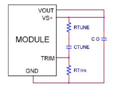
Figure. 3. Circuit diagram showing connection of RTUNE and CTUNE to tune the control loop of the module
