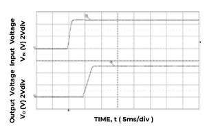
Figure 2. Typical Start-up using Input Voltage (Vin=12V, Vout = Vout, max, lout = lout, max)
