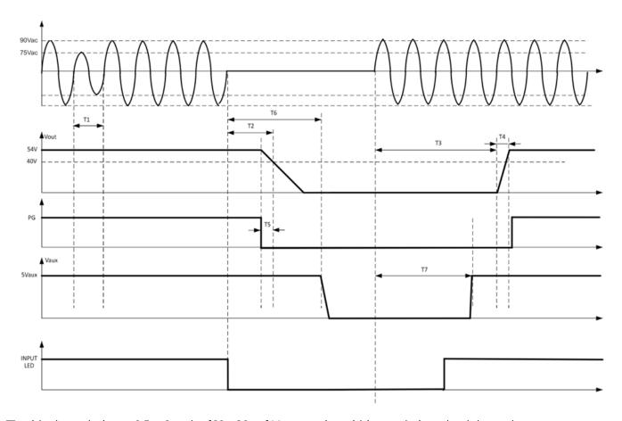
$\Pi$  - ride through time - 0.5 to 1 cycles [ 10 - 20ms]  $V_{OUT}$  remains within regulation - load dependent
