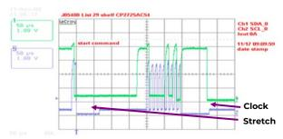
Example waveforms showing clock stretching.
