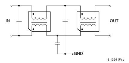
Figure 4. Internal Schematic
