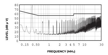
Figure 10.JAW075A1 Conducted Noise with Filter
