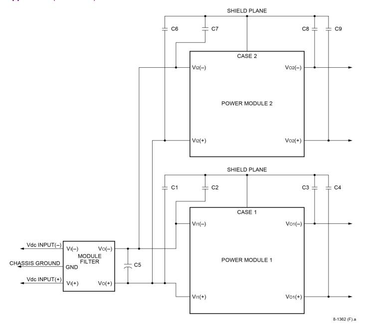
Note: C1 through C4 and C6 through C9 can be  $0.01\mu\text{F}$  to  $0.1\mu\text{F}$ . Select the voltage rating to meet input -to- output isolation requirements. C5 should be the recommended value indicated in the power module data sheet.
