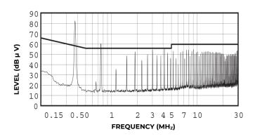
Figure 11.QHW100F1 Conducted Noise with Filter Compared to Class B Limits
