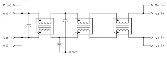
Figure 4. Internal Schematic
