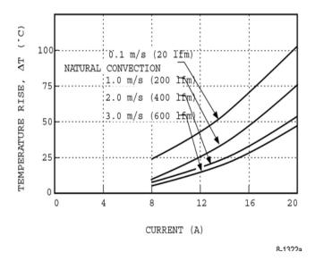
Figure 1. Typical Case Temperature Rise vs. Average Current (Case Temperature Must Be Kept Below  $100\ ^{\circ}\text{C}$ )
