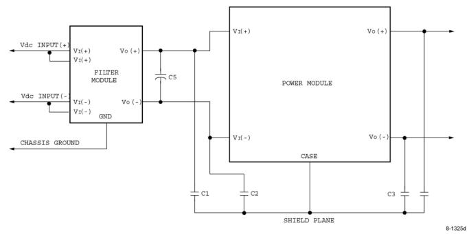
Note: C1 through C4 can be  $0.01\mu\text{F}$  to  $0.1\mu\text{F}$ . Select the voltage rating to meet input-to-output isolation requirements.C5 should be the recommended value indicated in the power module data sheet.
